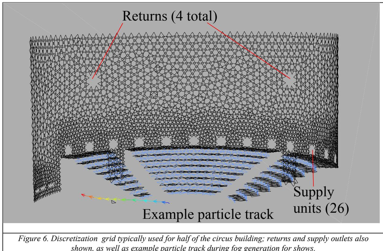
Figure 6. Discretization grid typically used for half of the circus building; returns and supply outlets also shown, as well as example particle track during fog generation for shows.
