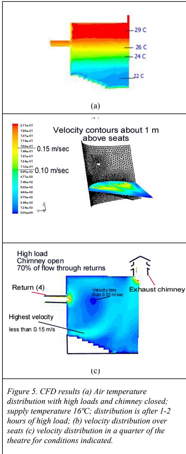
Figure 5. CFD results (a) Air temperature distribution with high loads and chimney closed; supply temperature 16°C; distribution is after 1-2 hours of high load; (b) velocity distribution over seats (c) velocity distribution in a quarter of the theatre for conditions indicated.
