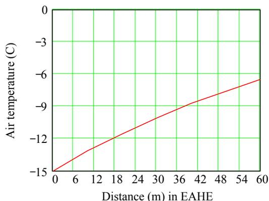
Figure 3b. Variation of air temperature in EAHE with distance from inlet in January ( $T_w = 3.3^\circ\text{C}$ ,  $T_o = -15^\circ\text{C}$ ).
