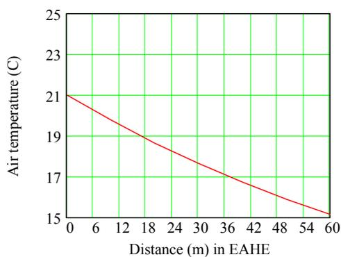
Figure 3a. Variation of air temperature in EAHE with distance from inlet ( $T_w = 8.4^\circ\text{C}$ ,  $T_o = 21^\circ\text{C}$ ).
