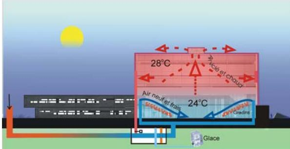
Figure 2. Schematic showing typical operation of hybrid ventilation system; fresh air is drawn from EAHE and exhausted from exhaust chimney or returns (four returns located at 17 m height).
