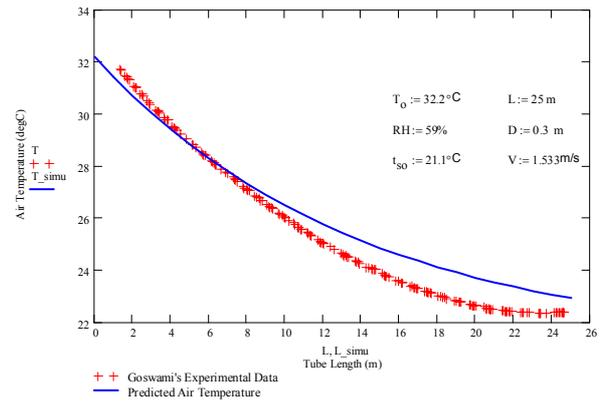
Figure 3. Comparison of EAHE model predictions with experimental data by Goswami et al. (1990) for a tube length of 25 m and 0.3 m diameter (soil temperature 21.1. C,  $V=1.533$  m/s).
