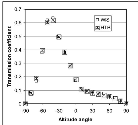
Figure 3; Comparison of total system transmission factor the W45 blind within a double glazed panel
