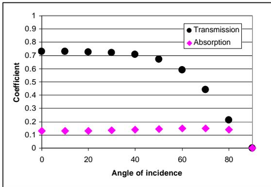
Figure 1; Graphical representation of an original HTB2 glazing characteristic of a 4mm float double glazing unit.
