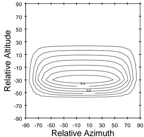
Figure 2; Graphical representation of a “2-D” HTB2 glazing transmission characteristic for a double glazing unit of 4mm float glass with horizontal slatted blinds.
