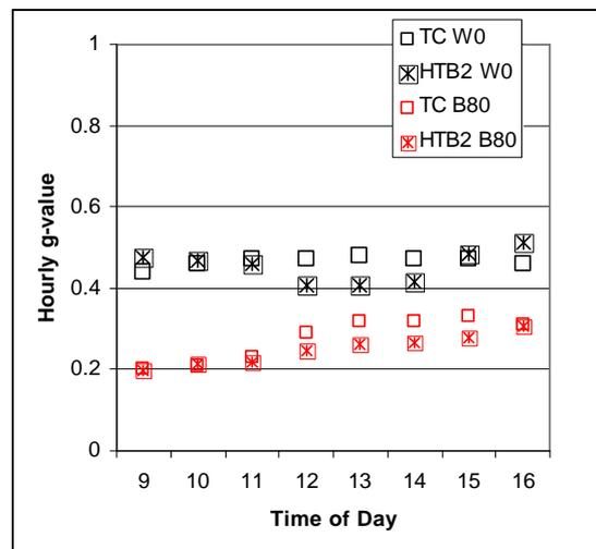
Figure 4; Comparison of hourly system  $g_d$ -value for two blind configurations; TC – measured data, HTB2 – simulations
