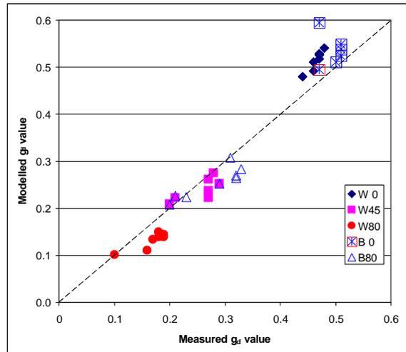
Figure 6; Comparison of all hourly system  $g_d$  - values, modified algorithms and 5 degree tables.
