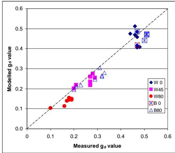
Figure 5; Comparison of all hourly system  $g_d$  - values, original model algorithms
