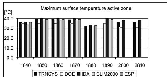
Figure 6: Maximum floor surface temperature for cases 1840 to 2810
