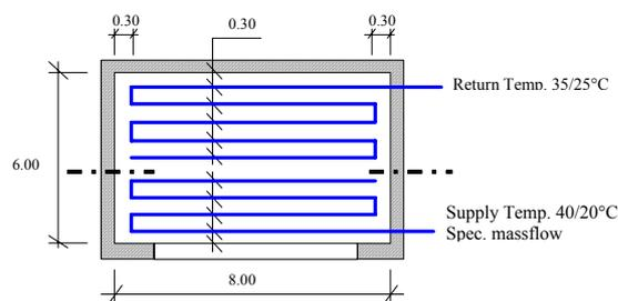
Figure 3: Detailed description of radiative system
