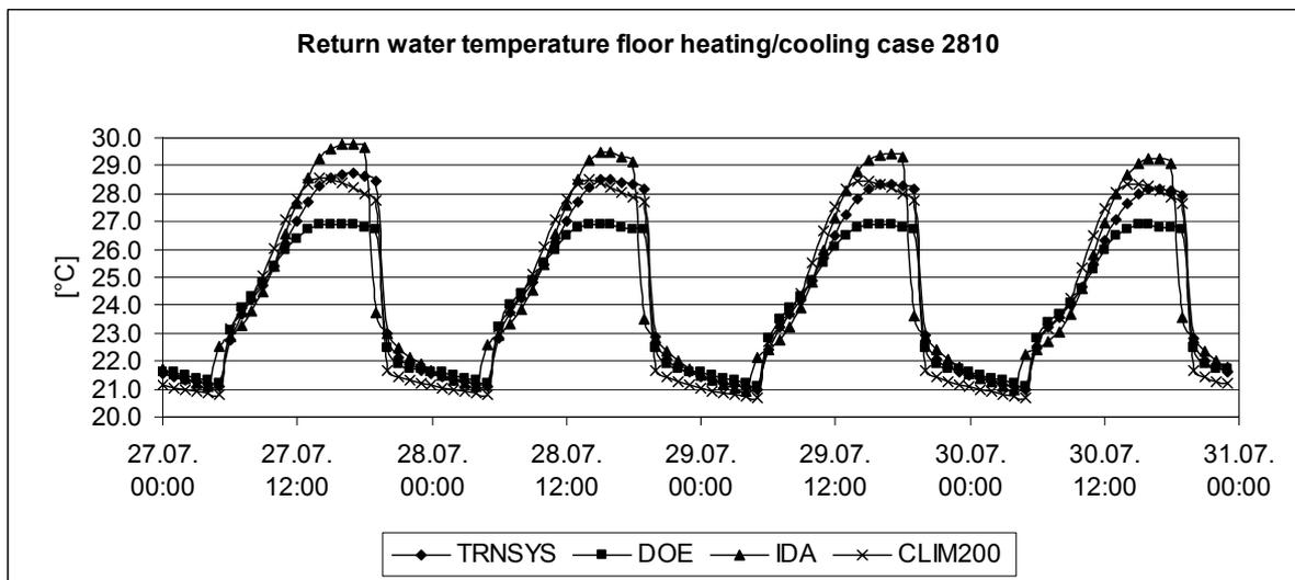
Figure 8: Return water temperature plot for a detailed water loop model
