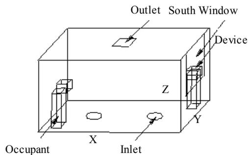
Figure 2. Configuration of the simulated office room
