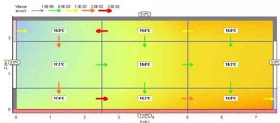
Figure 9: Temperature and mass airflow obtained with Sim\_zonal
