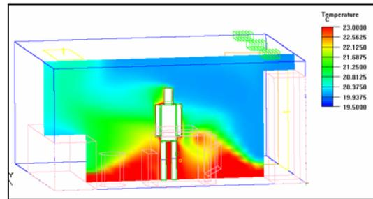
Figure 6: Temperature field obtained with Airpack
