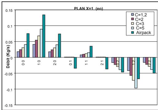
Figure 12: Mass airflow evolution with increasing of pressure coefficient
