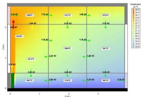
Figure 17: Temperature field in a room in case of fan cooler presence
