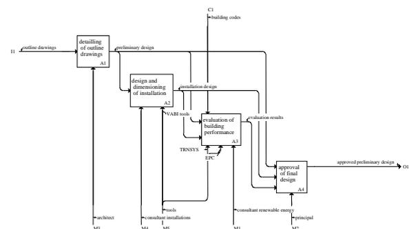
Figure 4: part of the process model describing the design process of ECN Building 42
