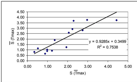
Figure 2. Correlation between the average of standard deviation of daily maximum temperatures ( $\bar{S}_{(Tmax)}$ ) and the standard deviation of the average of monthly maximum temperatures ( $S_{(\bar{T}_{max})}$ ), for 14 Brazilian cities.
