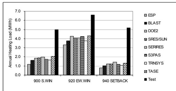
Figure 8. High mass annual heating load (MWh)
