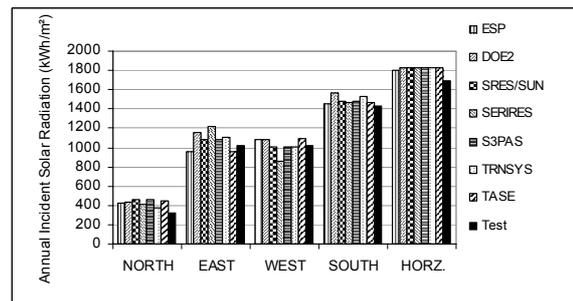
Figure 12. Annual incident solar radiation (kWh/m<sup>2</sup>)
