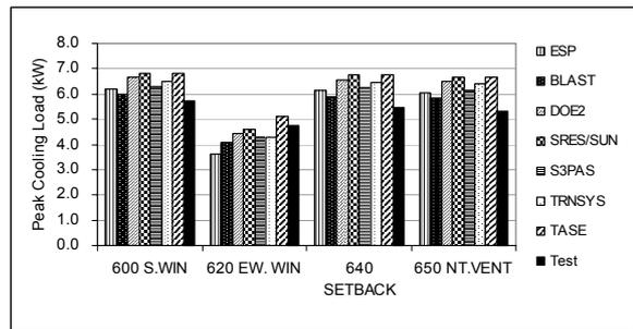
Figure 7. Low mass peak cooling load (kW)
