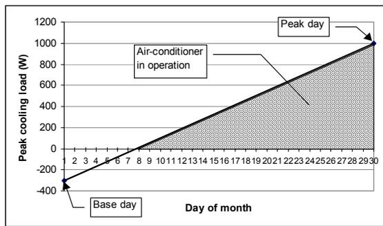
Figure 1. Days with air conditioning systems running in a generic month, between two typical days.
