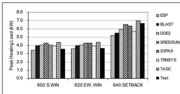
Figure 6. Low mass peak heating load (kW)
