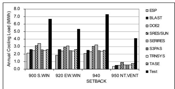
Figure 9. High mass annual cooling load (MWh)
