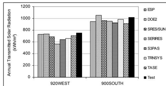
Figure 13. Annual transmitted solar radiation (kWh/m<sup>2</sup>)
