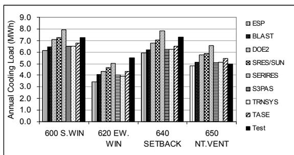
Figure 5. Low mass annual cooling load (MWh)
