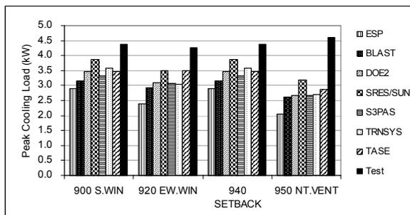
Figure 11. High mass peak cooling load (kW)
