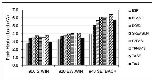
Figure 10. High mass peak heating load (kW)
