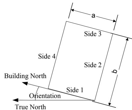
*Figure 2 Definition of orientation and aspect ratio*
