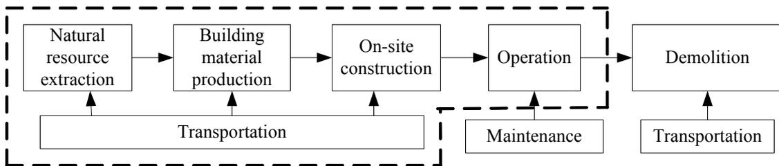
Figure 1 Building life-cycle process
