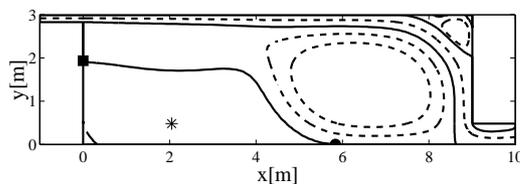
Figure 12: Flow structure for 2-D simulation using the  $k-\omega$  SST model. Symbols as in figure 9.
