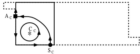
Figure 13: Topology in Annex 20 room. The sketch is based on 2-D simulations.
