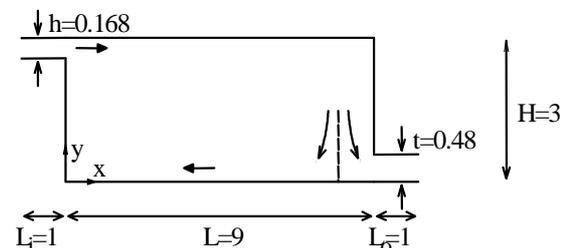
Figure 1: The isothermal Annex 20 room. The inlet and outlet were included in the original test case
