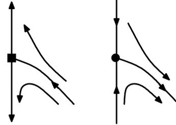
Figure 3: Left: Attachment point, ■, located on a vertical wall. Right: Separation point, ●, located on a vertical wall.
