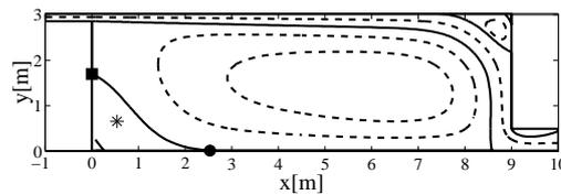
Figure 10: Flow structure for 2-D simulation using the  $k-\omega$  model. Symbols as in figure 9.
