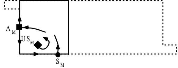
Figure 7: Topology in the symmetry plane of the Annex 20 room. The sketch is based on experiments in a water scale model.
