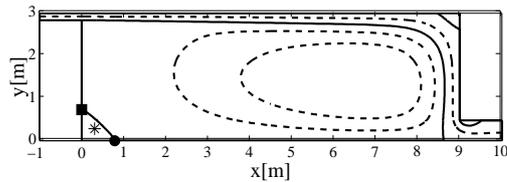
Figure 9: Flow structure for 2-D simulation using the  $k-\epsilon$  model.  $\bullet$ : Separation point.  $\blacksquare$ : Attachment point.  $*$ : Centre
