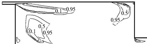
Figure 14: Value of the blending function appearing in the  $k-\omega$  BSL model. The value should be one near surfaces and zero away from surfaces.
