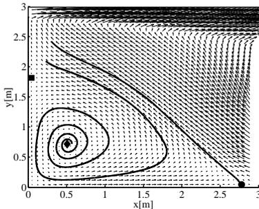
Figure 6: Ensemble averaged velocity vector field in the symmetry plane of the Annex 20 room. Solid
