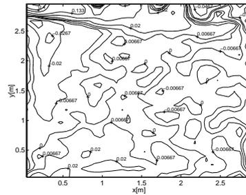
Figure 8: Contours of  $-\partial w / \partial z$  calculated from the continuity equation.
