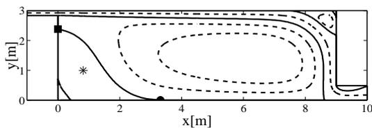
Figure 11: Flow structure for 2-D simulation using the  $k-\omega$  BSL model. Symbols as in figure 9.
