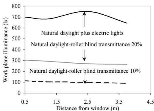
Fig. 7. Illuminance distribution on the work plane in a typical office on SW façade (December 15<sup>th</sup>, afternoon).
