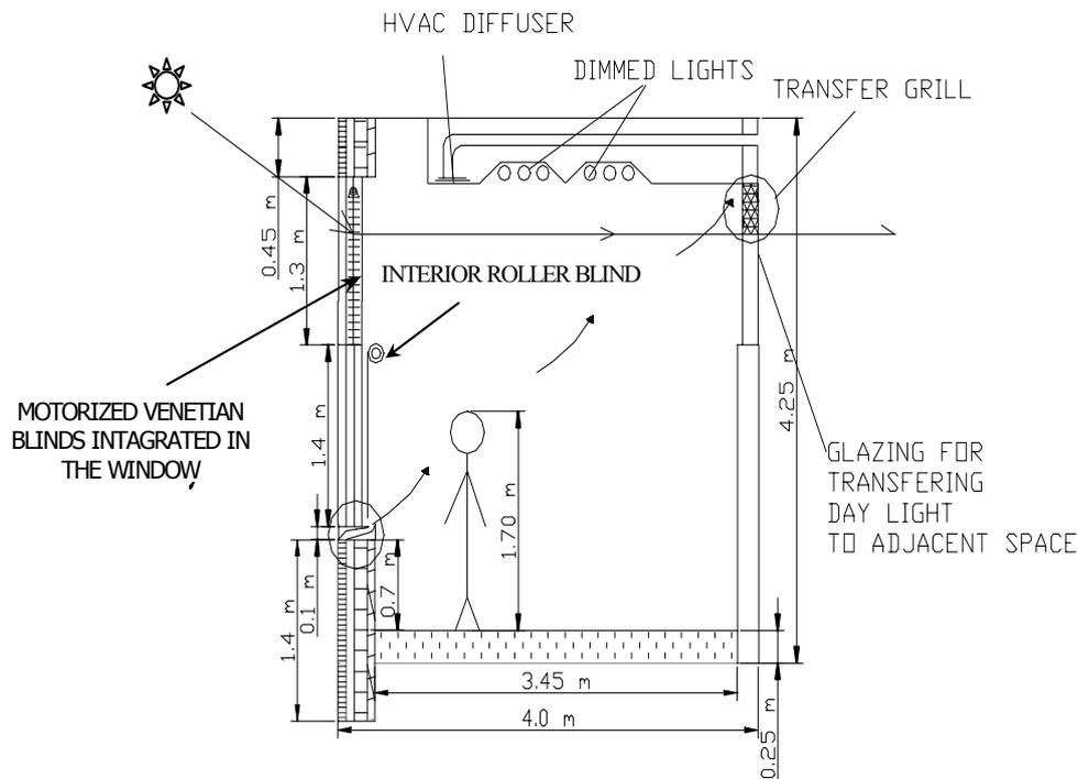
Fig. 5. A multifunctional façade with optimum shading and daylighting options for a typical perimeter office. The top part of the window consists of motorized venetian blinds and the bottom half is a manually controlled interior roller blind.
