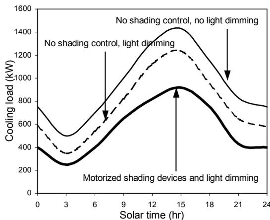
Fig. 9. Impact of light dimming and motorized shading on cooling load during a hot summer day.
