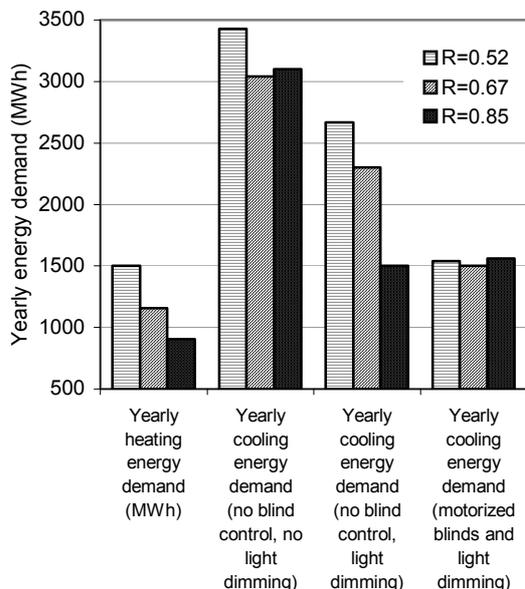
Fig. 10. Impact of glazing thermal resistance, blind control and light dimming on annual heating and cooling energy consumption (perimeter floor area is 5000 m<sup>2</sup>).
