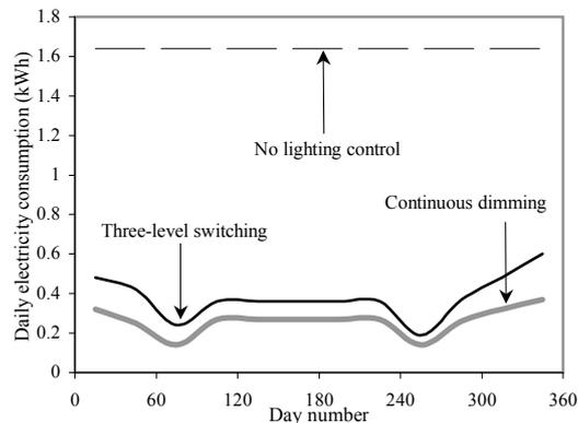
Fig. 6. Comparison of mean daily electricity consumption for lighting using continuous dimming, three-level switching and no lighting control in a typical office on SW façade.
