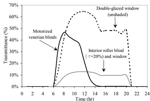
Fig. 1. Transmittance of window/shading device as a function of time (clear summer day).
