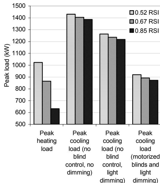
Fig. 8. Peak heating and cooling loads for different glazing R-values and the effect of blinds control and light dimming (perimeter floor area is 5000 m<sup>2</sup>).
