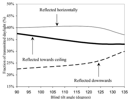
Fig. 2. Directional distribution of transmitted daylight through motorized venetian blinds, for different blind tilt angles ( $90^\circ$  is horizontal).
