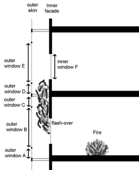
Figure 1: Double skin façade. In case of flashover, the outer windows B, C, D and E are obstructing the flame geometry. Window A is not obstructing the flame and can be neglected.
