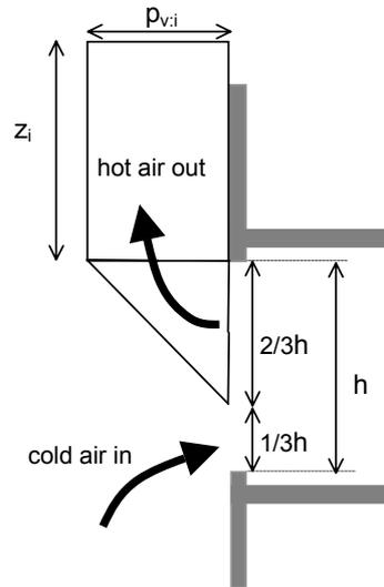
Figure 3: shape of flame according to the NEN 6068 (no obstructions)
