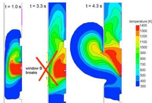
Figure 7: results of CFD-model, snapshots at  $t = 1.0$  s,  $t = 3.3$  s and  $t = 4.3$  s. Note that window B breaks at  $t = 3.3$  s.
