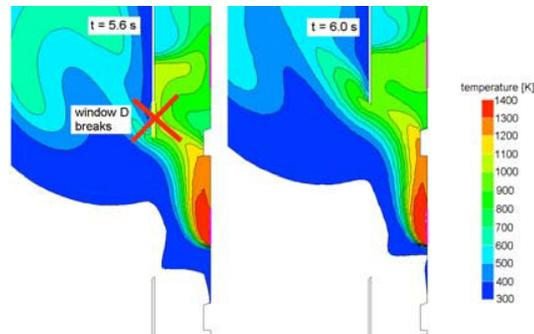
Figure 9: results of CFD-model, snapshots at  $t = 5.6$  s and  $t = 6.0$  s. Note that window D breaks at  $t = 5.6$  s.
