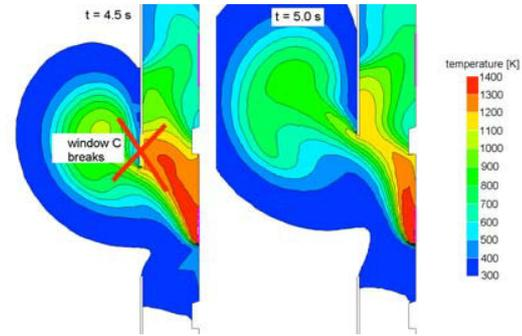
Figure 8: results of CFD-model, snapshots at  $t = 4.5$  s and  $t = 5.0$  s. Note that window C breaks at  $t = 4.5$  s.
