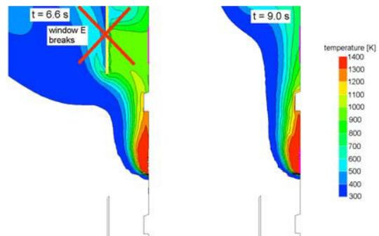
Figure 10: results of CFD-model, snapshots at  $t = 6.6$  s and  $t = 9.0$  s. Note that window E breaks at  $t = 6.6$  s.
