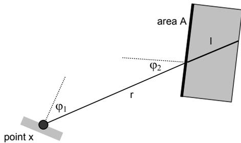
Figure 5: the configuration factor which is determined by  $\phi_1$  and  $\phi_2$ .
