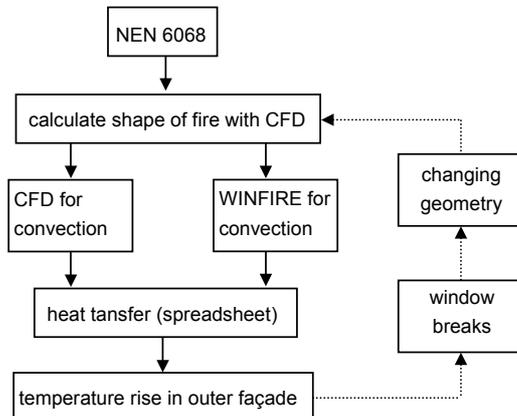
Figure 2: flow diagram of the simulation
