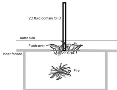
Figure 4: the 2D fluid domain region used for CFD.
