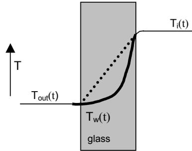
Figure 6: Profile of the temperature in the glass for steady state situation (dotted line) and transient situation (solid line).
