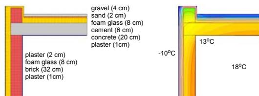
Figure 13. Cross-section and typical temperature profile for corner solution with insulated brick exterior wall.
