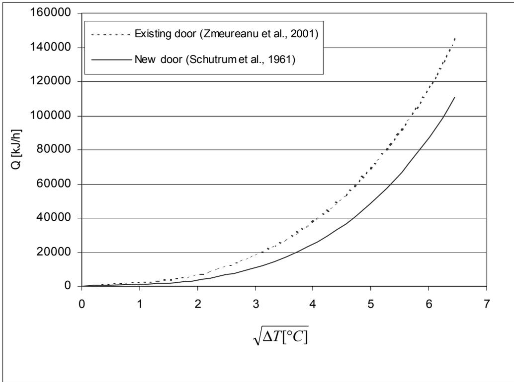
Figure 6: Estimated heat loss due to air infiltration versus temperature difference. Comparison between an existing door (Zmeureanu et al., 2001) and a new door (Schutrum et al., 1961).
