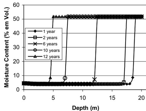
Figure 9. Moisture Content profiles of the sandy silt soil considering water table as the bottom surface boundary condition.
