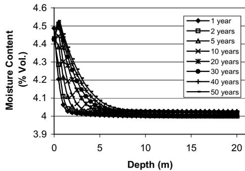
Figure 5. Moisture content profiles of the sandy silt soil at 12 pm on December 31<sup>st</sup>.
