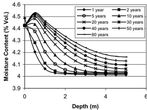
Figure 7. Moisture content profiles in a soil physical domain with a 5-m depth.
