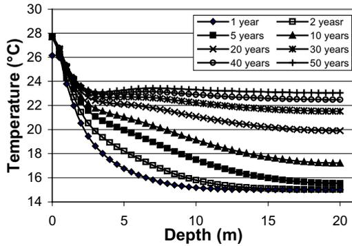
Figure 4. Temperature profiles of the sandy silt soil at 12 pm on December 31<sup>st</sup>.
