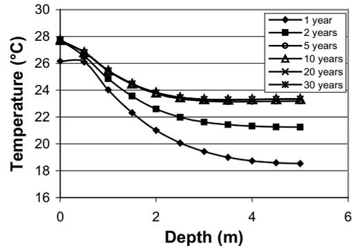
Figure 6. Temperature profiles in a soil physical domain with a 5-m depth.
