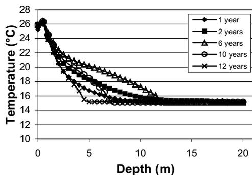
Figure 8. Temperature profiles of the sandy silt soil considering water table as the bottom surface boundary condition.
