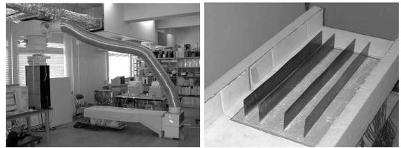
(a) Experiment Space (b) Fin Embedded Concrete
