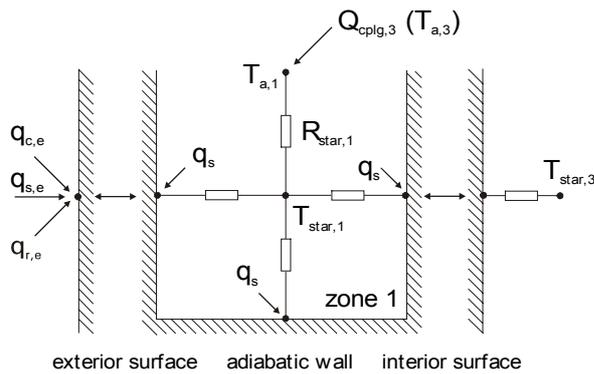
**Figure 7:** Representation of the inlet zone as a separate zone in a building energy simulation program.
