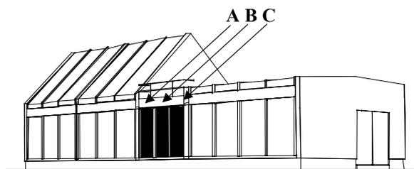
**Figure 4:** The Vliet test building experimental setup: (A) classical cladding system, (B) mechanically ventilated facade, (C) naturally ventilated facade.
