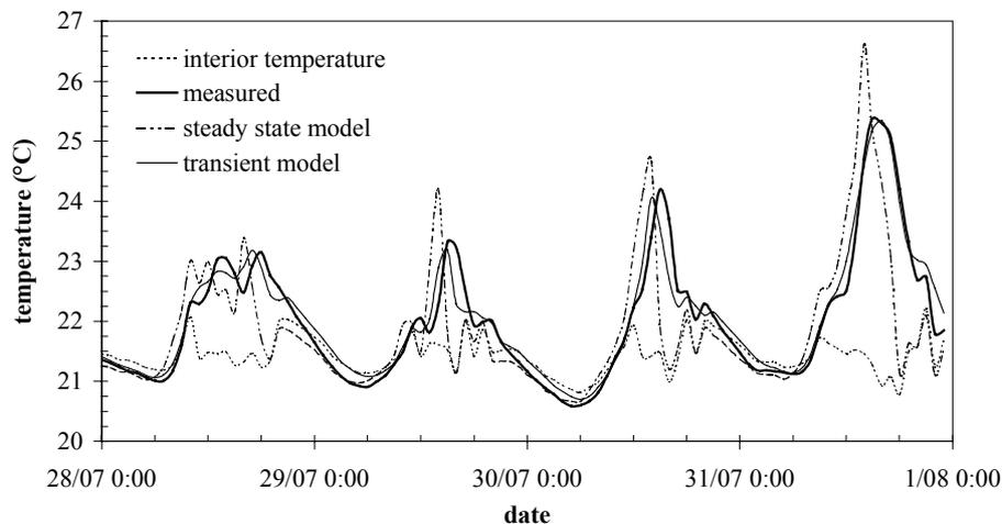
**Figure 8:** Comparison of the measured inlet temperature with the inlet temperature as calculated by the steady state and transient model. for an airflow window ( $G_a = 37 \text{ m}^3/\text{h}$ ).
