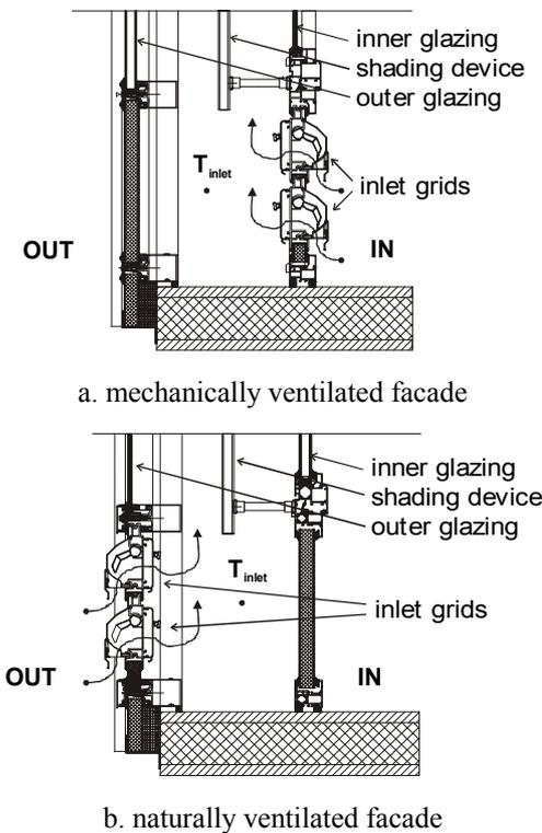
**Figure 5:** Construction details of the inlet zone of the mechanically and naturally ventilated MSF.
