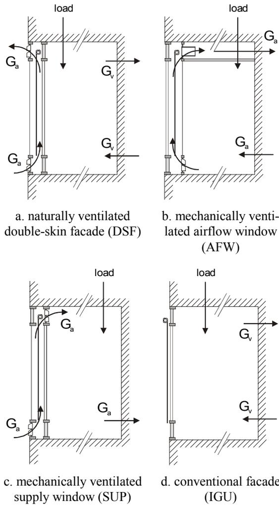
**Figure 9:** Diagram of the simulated multiple-skin facades;  $G_a$  represents the airflow rate through the multiple-skin facade cavity,  $G_v$  is the minimum hygienic ventilation rate.
