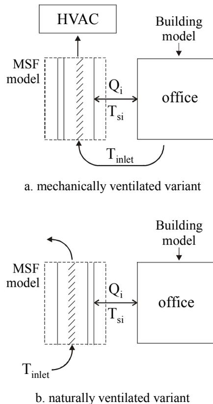
**Figure 1:** Typical implementations to calculate the energy performance of multiple-skin facades.
