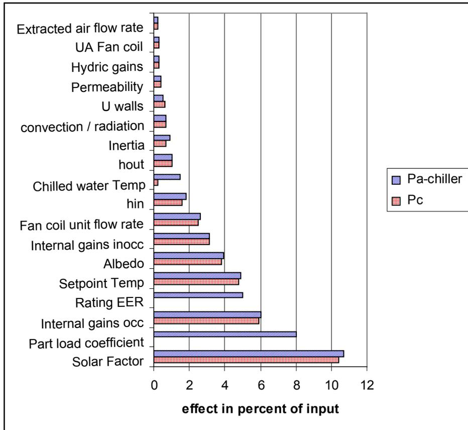
Figure 4 Simple effects on chiller cooling power and electrical input power
