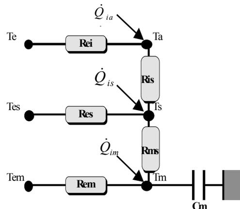
Figure 1 Equivalent electric representation of the building model
