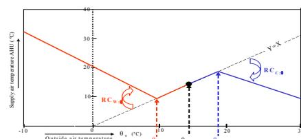
Figure 4: Optimised heating/cooling curve.
