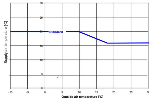
Figure 1: Standard heating/cooling curve for AHU
