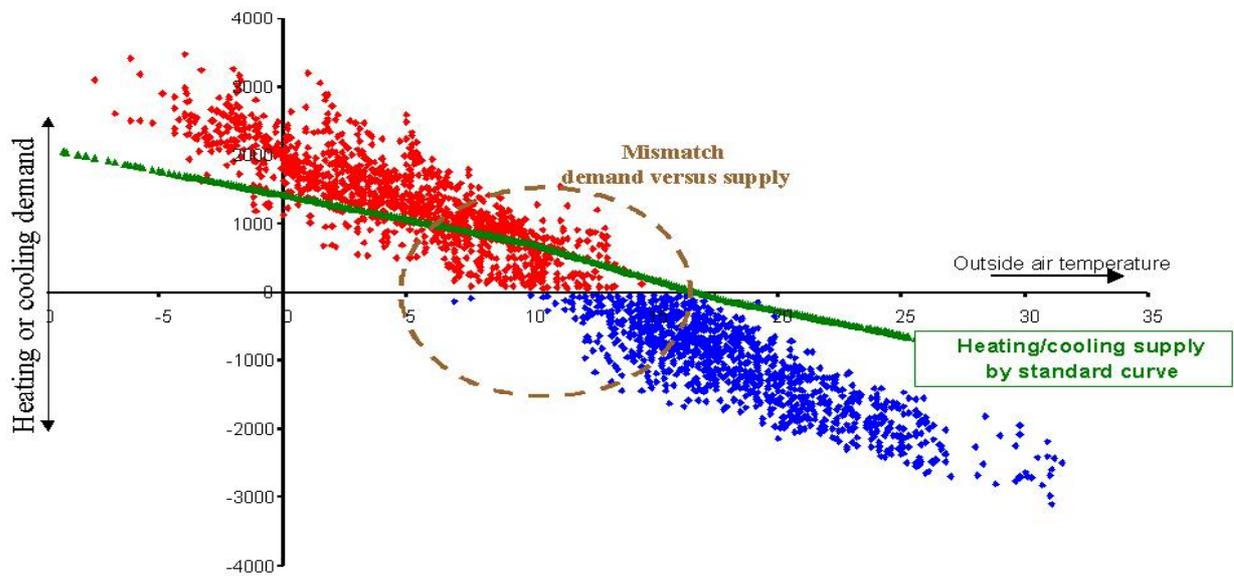
Figure 2: Energy demand profile showing energy mismatch due to standard heating/cooling curve
