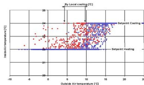
Figure 9: Improved comfort through adjusting the heating /cooling curve
