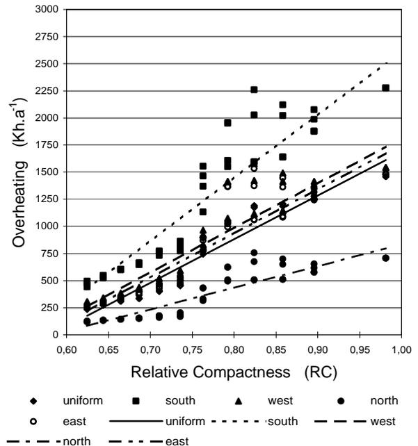
Figure 10 – Simulated overheating as a function of RC and glazing distribution options (all instances with 40% glazing)
