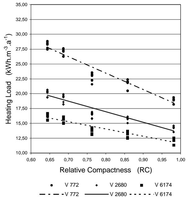
Figure 16 – Heating load of sample C as a function of RC (for three volume ranges and 25% glazing option)
