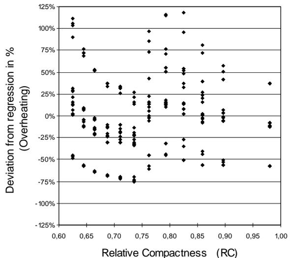
Figure 12 – Deviation of simulated overheating results from regression-based predictions (for 40% glazing option)
