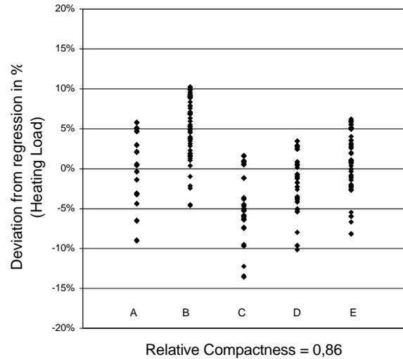
Figure 14 – Deviation of simulated heating loads (for the sample of five shapes with identical RC values) from regression-based predictions of the original sample (cp. Figure 6)
