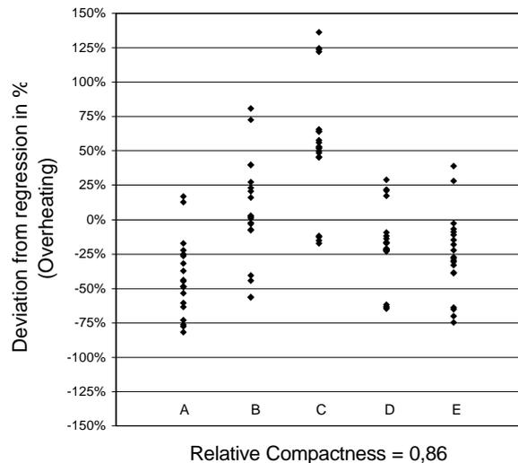
Figure 15 – Deviation of simulated overheating results (for the sample of five shapes with identical RC values) from regression-based predictions of the original sample (cp. Figure 9)
