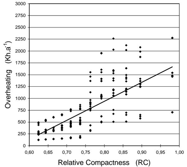
Figure 9 – Simulated overheating as a function of RC (all instances with 40% glazing)
