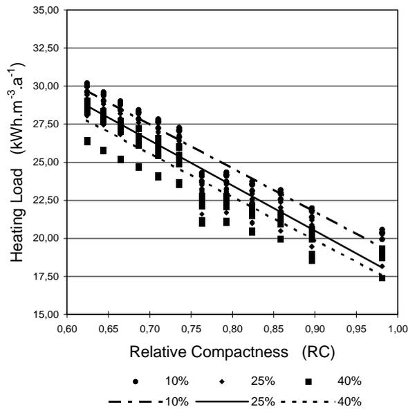
Figure 7 – Simulated heating loads as a function of RC and glazing percentage (10%, 25%, and 40%)
