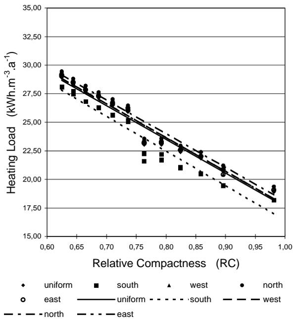
Figure 8 – Simulated heating loads as a function of RC and glazing distribution options (for 25% glazing option)
