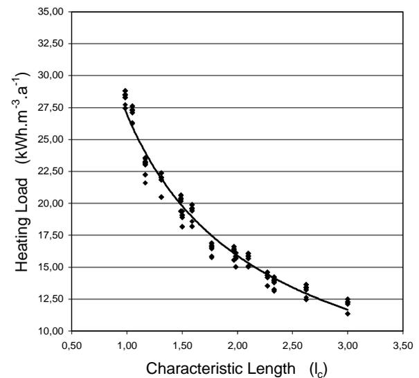
Figure 17 – Heating load of sample C as a function of  $l_c$  (for the 25% glazing option)
