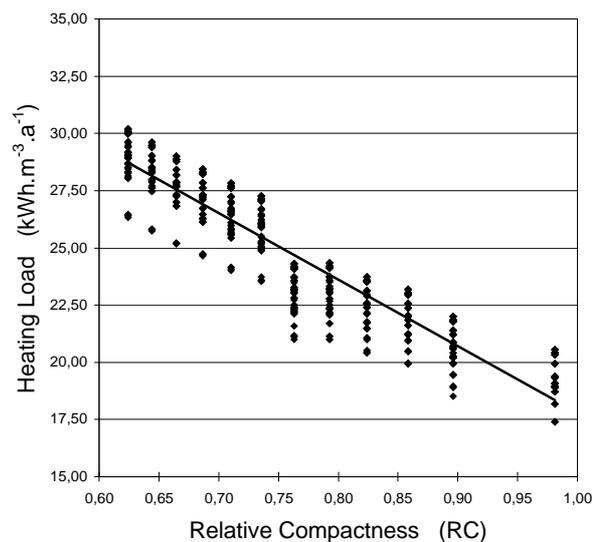
Figure 6 – Simulated heating loads as a function of RC (all instances)
