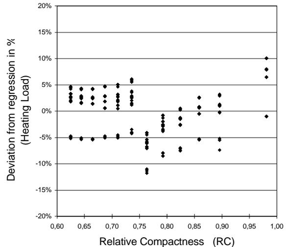
Figure 11 – Deviation of simulated heating loads from regression-based predictions (for 40% glazing option)
