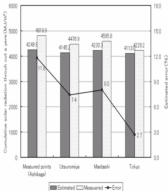
Figure 6. Estimated and measured cumulative global irradiance over a year
