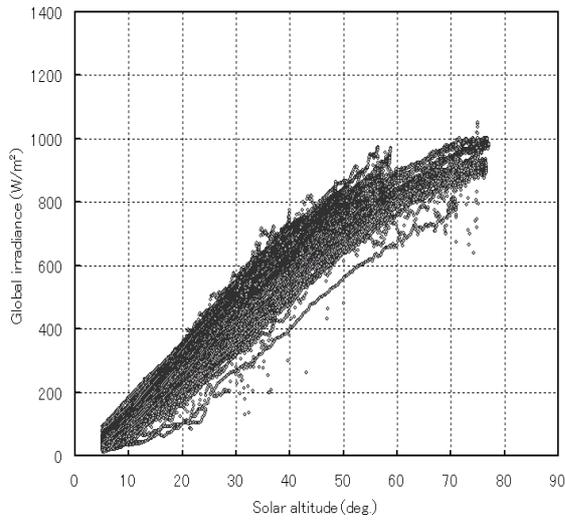
Figure 2. Measured data for the Clear sky conditions
