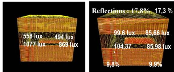
Figure 7: a) Lighting of the office cell working plane considering the walls and the slats reflections, b) Lighting of the office cell working plane due to the slats reflections.
