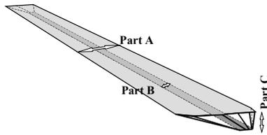
Figure 4: Slat optimal shape having a given thickness C. The A portion (upper part) of the strip alone gives the same protection than the B (lower part) and C (thickness) portions together.
