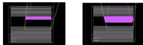
Figure 8: Electrochromic protection in the colored state during the day – working plane protected on June 21 from 3pm to 4pm (on the left) and on June 21 from 4pm to 5pm (on the right).
