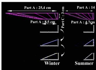
Figure 6: Slats optimal width and fall/winter and spring/summer options of slats shapes.
