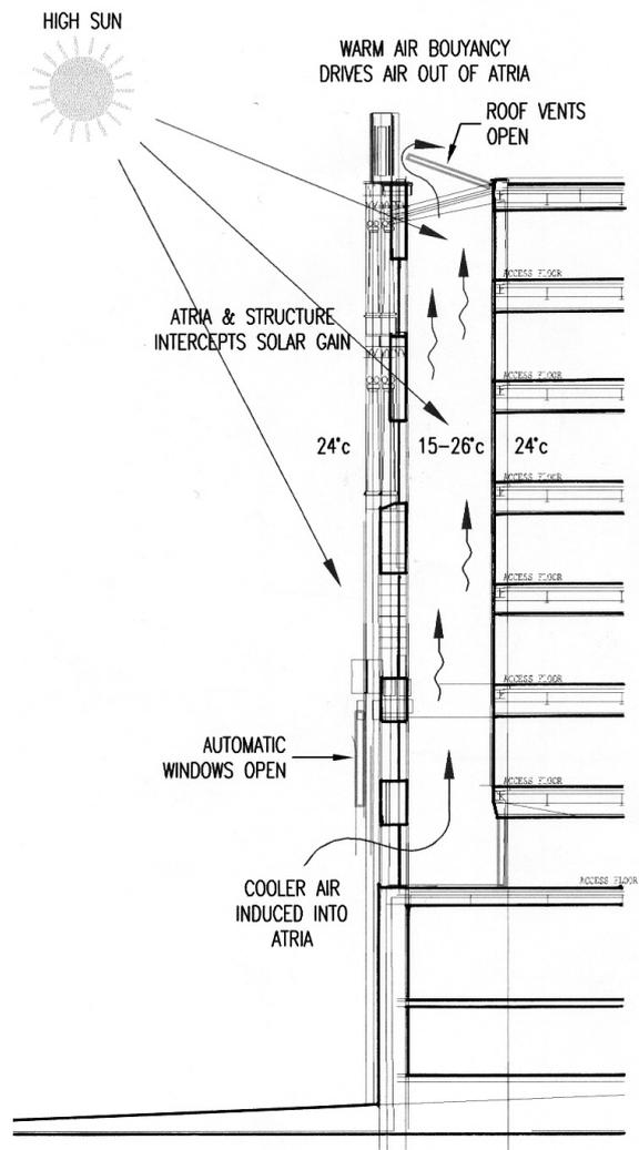
Figure 3: Typical buffer section.
