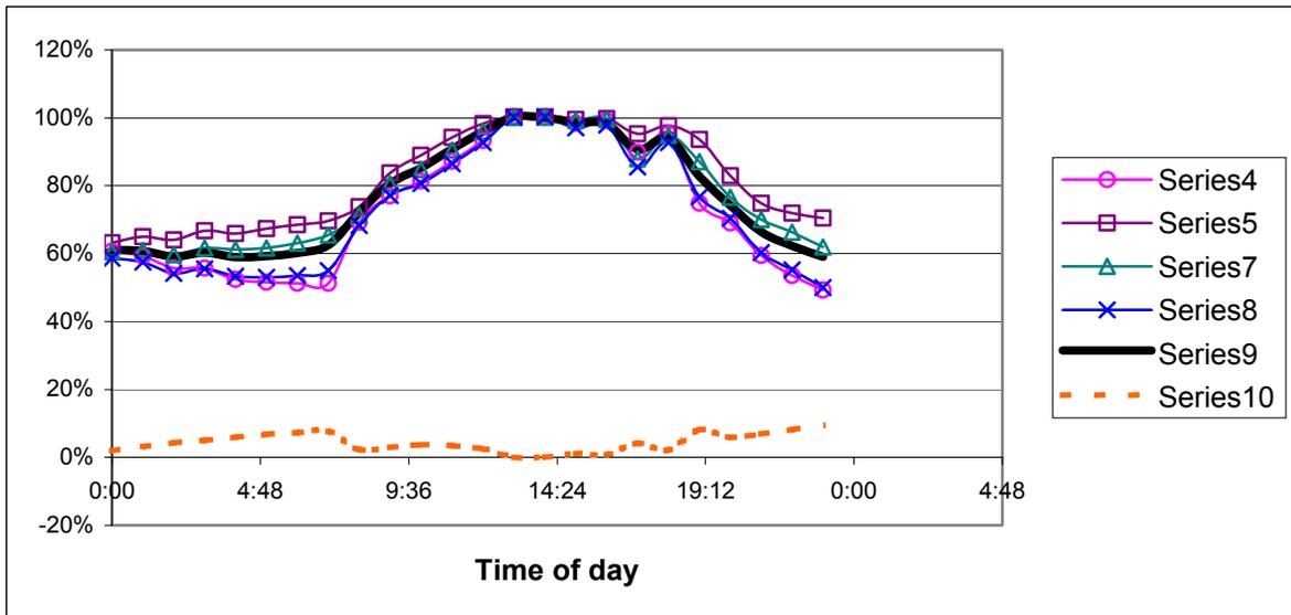
Figure 2 Cooling load profiles in July: S.4 – building weight 140 kg/m<sup>2</sup>; S.5 - building weight 590 kg/m<sup>2</sup>. Cooling load profiles in January: S.7- building weight 140 kg/m<sup>2</sup>; S.8- building weight 590 kg/m<sup>2</sup>; S.9 – average cooling load profile; S.10 – variance of the profiles
