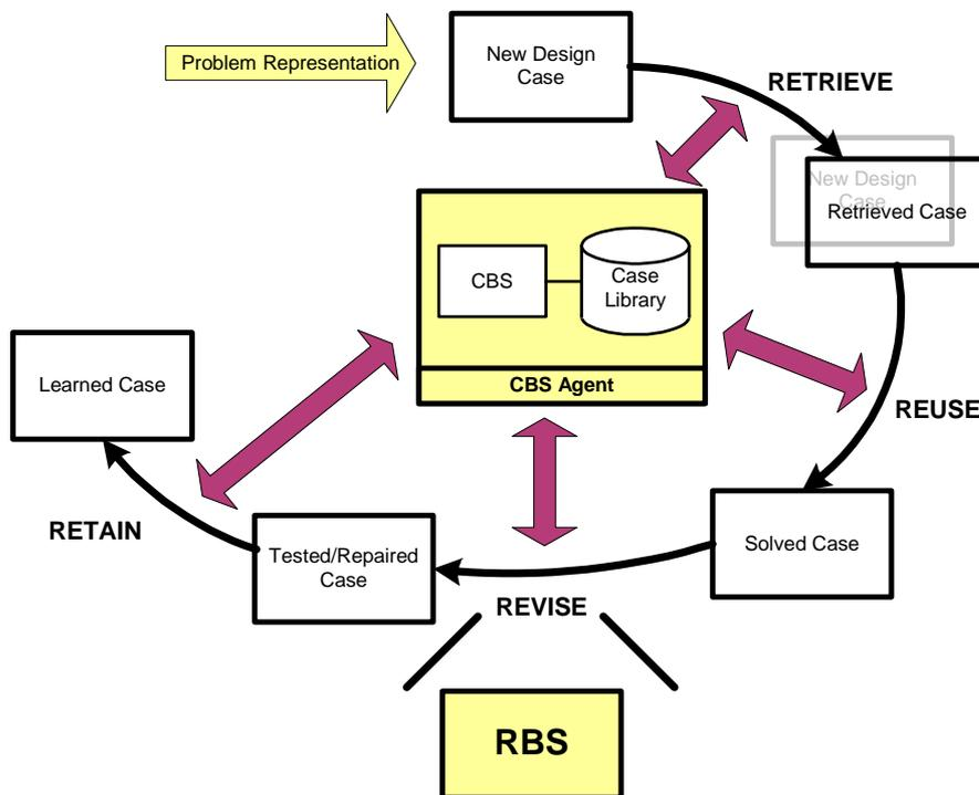
Figure 4 Method to use CBS to create a new design.
