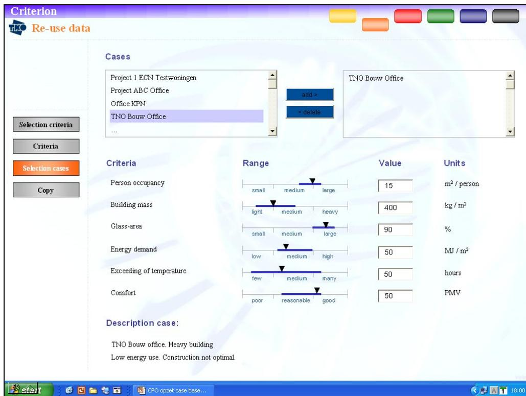
Figure 5 User interface: selection of design aspects from earlier design projects using the CBS with performance indicators.
