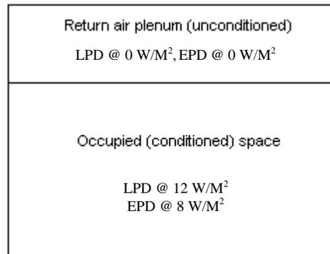
*Figure 2: Cross-section view of typical room showing conditioned and unconditioned spaces, with typical lighting power density (LPD) and equipment power density (EPD). The total internal heat gain from these sources totals 20 W/M<sup>2</sup>.*
