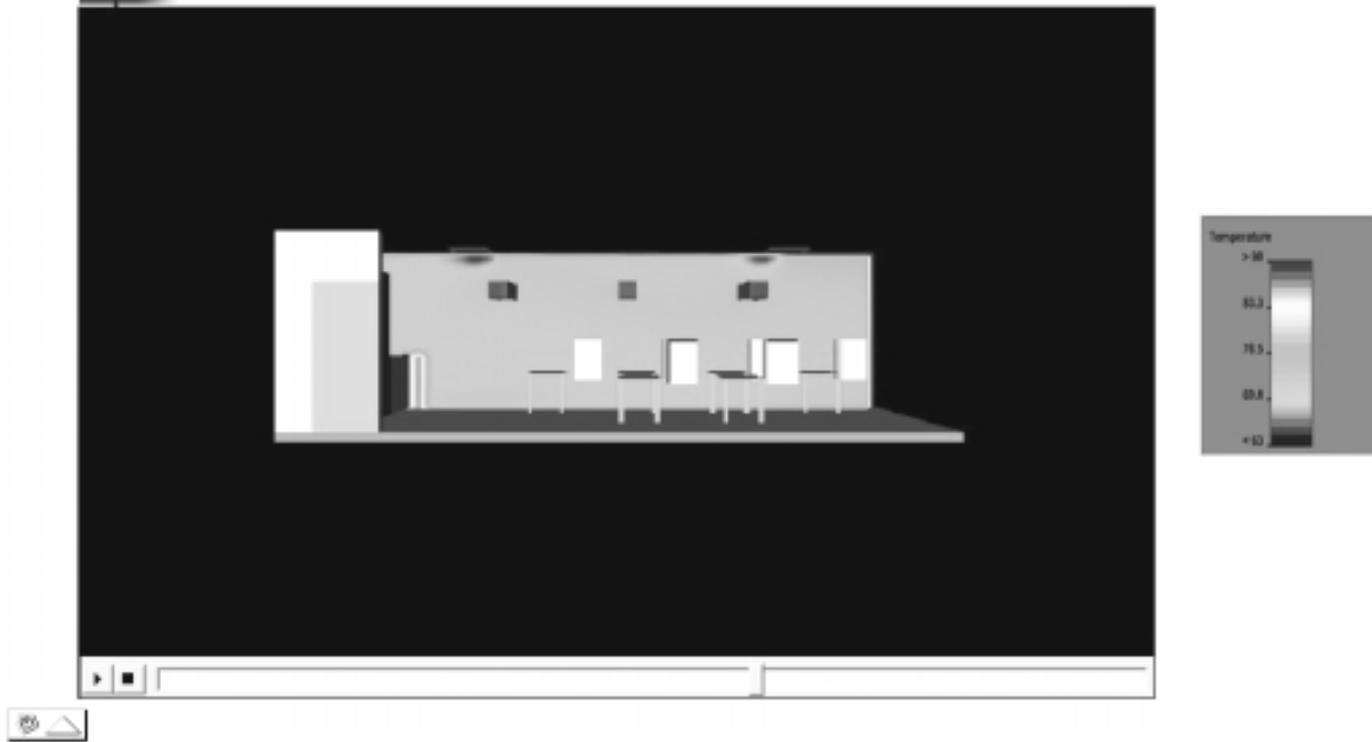
*Figure 5: Conventional Overhead Air Distribution System. This cross section of a 100 M<sup>2</sup> classroom CFD model of air temperature distribution predicts uniform space temperatures from floor to ceiling. The coolest temperatures are located at the supply air diffusers. The entire volume of the classroom is cooled to a comfortable temperature even though occupants only experience the thermal environment from floor level up to about 2 meters above the floor.*
