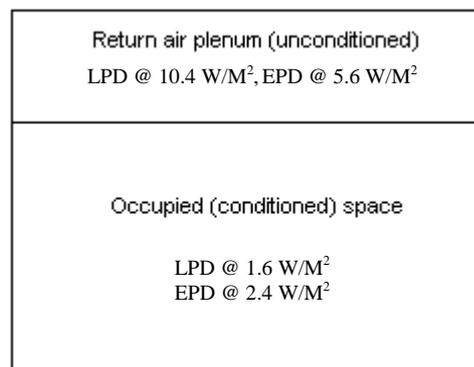
*Figure 3: To simulate the reduced heat gain from lighting and receptacle loads, much of the load is reassigned to the unconditioned return air plenum. The effect is that cooling loads in the conditioned space are reduced while the return air temperature is increased. The total gain from lights and plugs is unchanged, however, it has been apportioned differently between conditioned and unconditioned space.*
