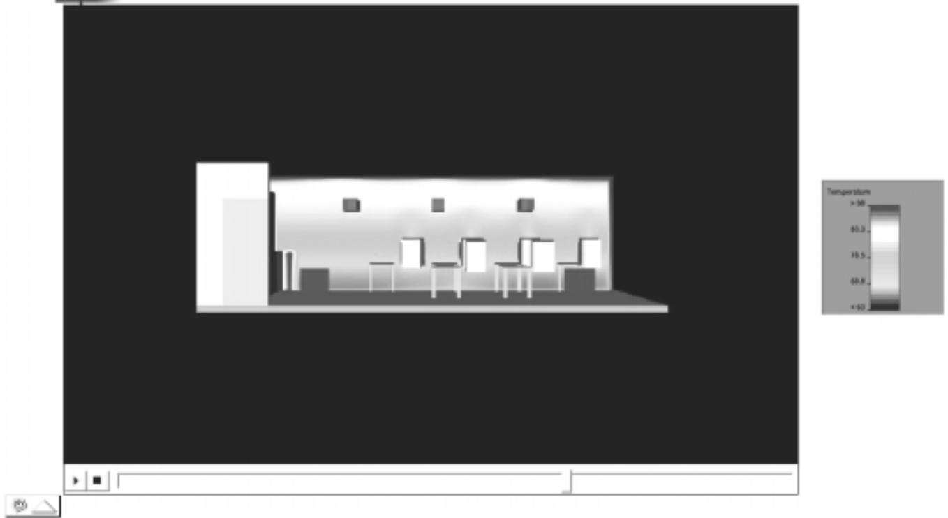
*Figure 6: Thermal Displacement Ventilation System. This cross section of a 100 M<sup>2</sup> classroom CFD model of air temperature distribution predicts that stratification occurs when air is supplied at floor level at a low velocity. Acceptable temperatures are found at the level of building occupants, whereas there is a layer of very warm air located just below the ceiling.*
