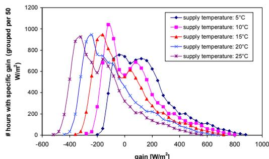
Figure 10. Yearly number of hours of a specific heat gain as function of the supply temperature (15 mm wearing course).
