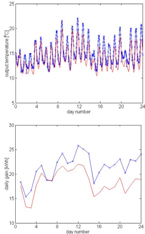
Figure 6. Measured + simulated output temperature and daily energy gain of the asphalt collector (2½-D model; [-] measurement, [x] simulation).
