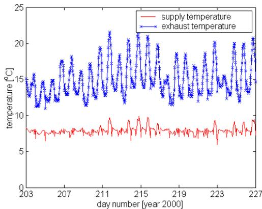
Figure 4. Supply and exhaust temperature of the heat exchanger over a period of 3.5 weeks.
