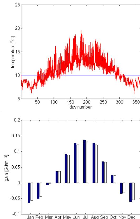
Figure 7. The calculated output temperature of the asphalt collector (top; 2½-D model) and the monthly thermal energy gain (bottom; closed: 2½-D model, open: 1½-D model).
