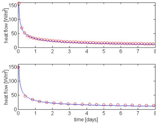
Figure 5. Result analytical validation (top: 2½-D-model, bottom: 1½-D model; line: analytical result).
