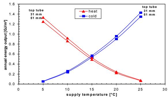
Figure 8. Annual thermal energy gain as a function of the supply temperature and depth of tubes.
