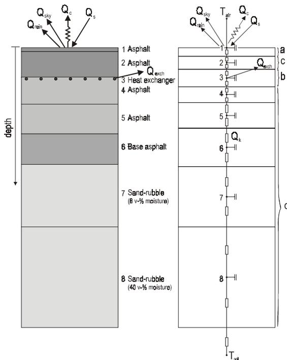
Figure 2. Schematic representation of the design of an asphalt collector and the derived network model.
