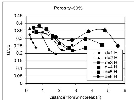
Figure 8. The wind curves of speed with different distance ( $d$ ) between windbreak and building (wind tunnel experiment; the windbreaks stand at  $x=0.0$ , the buildings stand at the  $x$  position of the end of each curve respectively).
