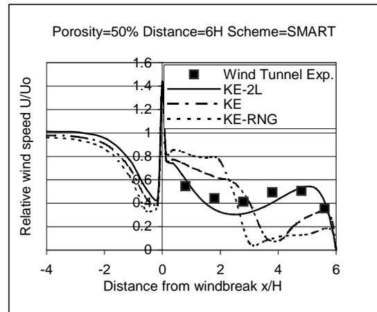
Figure 3. Mean horizontal wind speed ratio at the ground level (Comparison about different turbulence models application;  $d=6H$ ).
