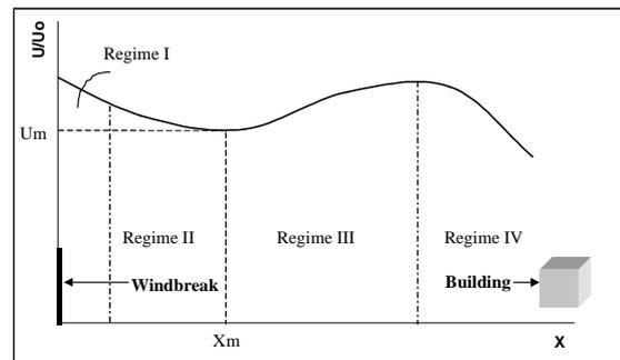
Figure 7. The flow regimes behind the windbreak with building in certain distance (this study).
