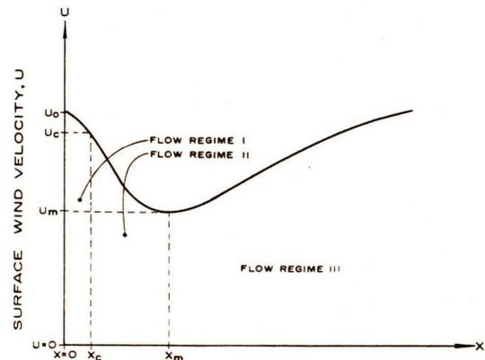
Figure 6. The flow regimes behind the windbreak (Bean 1975) ( $U_m$ -- The minimum mean wind speed.  $x_m$ -- the  $x$  position of the minimum wind speed).
