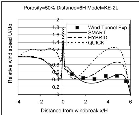
Figure 5. Mean horizontal wind speed ratio at the ground level (Comparison about different discretization schemes application;  $d=6H$ ).
