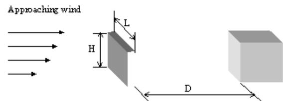
Figure 2. The layout of the building and windbreak ( $L$ —Length,  $H$ —Height,  $D$ —Distance)
