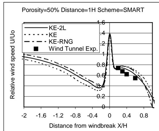
Figure 4. Mean horizontal wind speed ratio at the ground level (Comparison about different turbulence models application;  $d=1H$ ).
