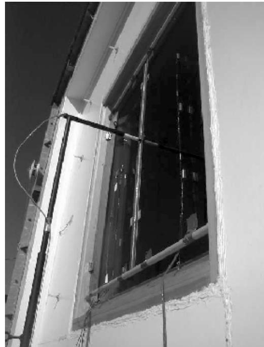
Figure 4: Prototype of the SOLVENT window (in summer mode) installed at the PASSYS test cell.
