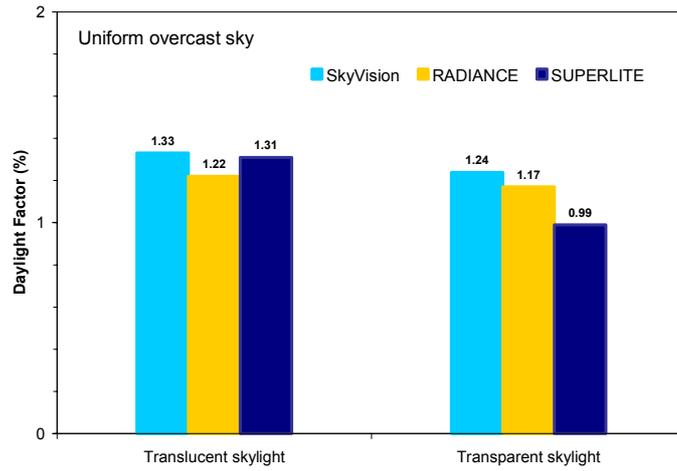
Figure 6: Comparison of the average Daylight Factor at floor level under a uniform overcast sky condition – case 2 (indoor space with 6.25% glazed roof and a light well)
