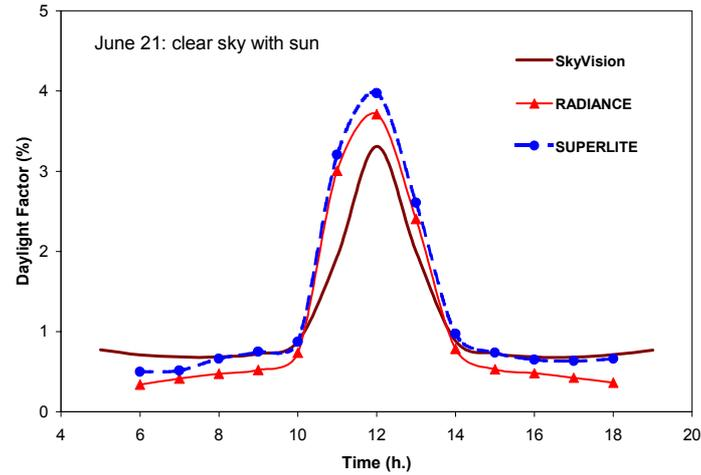
Figure 8: Comparison of the average Daylight Factor at floor level under a clear sky with sun condition – case 2 (indoor space with 6.25% glazed roof and a light well).
