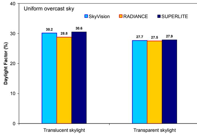
Figure 3: Comparison of the average Daylight Factor at floor level under a uniform overcast sky – case 1 (indoor space with 100% glazed roof and without a light well)
