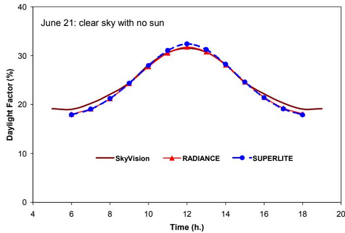
Figure 4: Comparison of the average Daylight Factor at floor level under a clear sky without sun – case 1 (indoor space with 100% glazed roof and without a light well)
