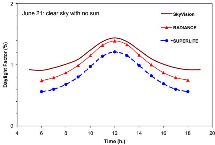
Figure 7: Comparison of the average Daylight Factor at floor level under a clear sky without sun condition– case 2 (indoor space with 6.25% glazed roof and a light well)
