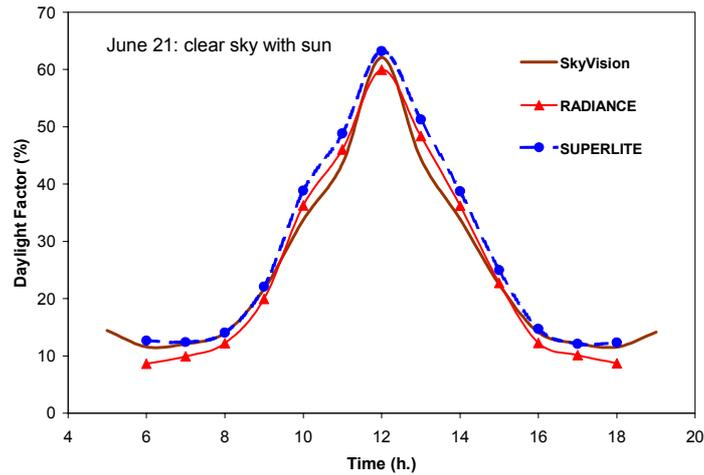
Figure 5: Comparison of the average Daylight Factor at floor level under a clear sky with sun – case 1 (indoor space with 100% glazed roof and without a light well).
