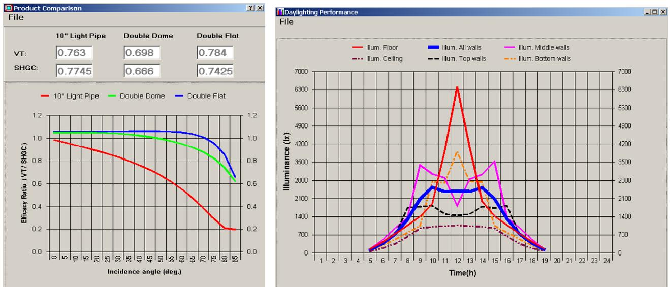
Figure 2: Typical output results: Skylight optical characteristics comparison and illuminance distribution on indoor surfaces
