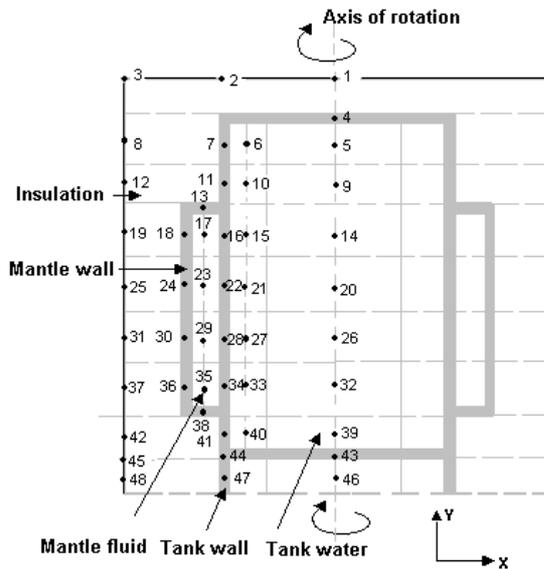
Figure 2 Numerical mantle tank model
