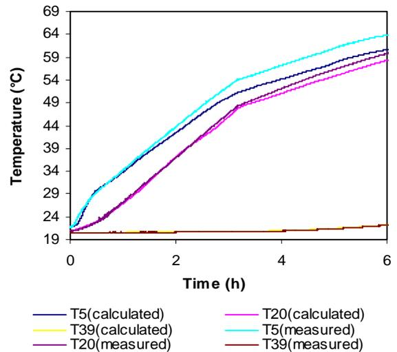
Figure 8 Variation of three temperatures calculated and measured in the storage tank for injection of the fluid at different levels in the mantle with electric supply.
