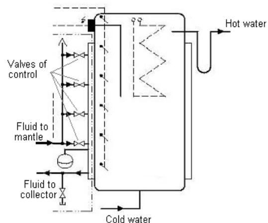
*Figure 1 Mantle solar tank with injection at several levels.*
