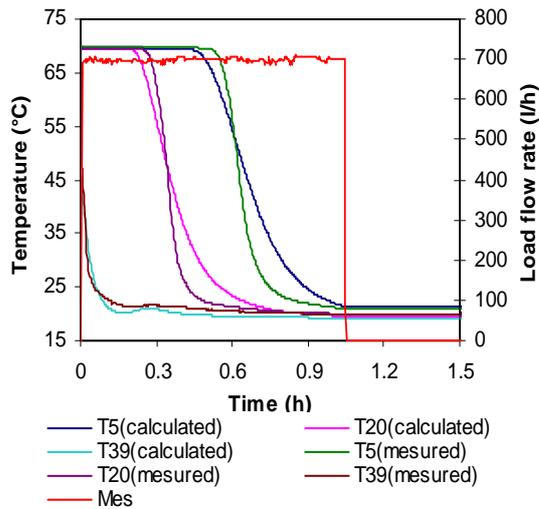
Figure 10 Variation of three temperatures calculated and measured in the storage tank for a step of load flow rate.
