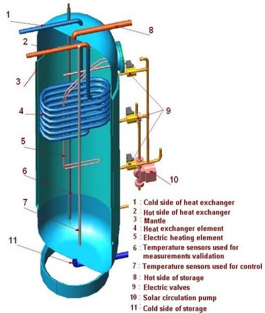
Figure 5 A vertical section of the instrumented storage tank
