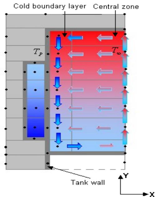
Figure 3 Exchange diagram relative to different zones where ( $T_p < T_\infty$ ).
