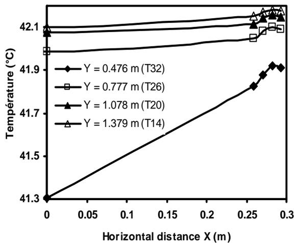
Figure 7 Temperature variation of the top part of the tank and its mantle according to X (radius) at different levels of the tank.
