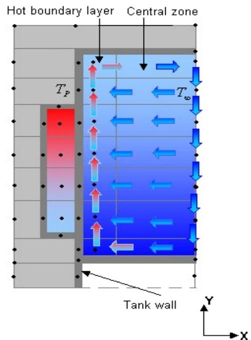
Figure 4 Exchange diagram relative to different zones where ( $T_p > T_\infty$ ).
