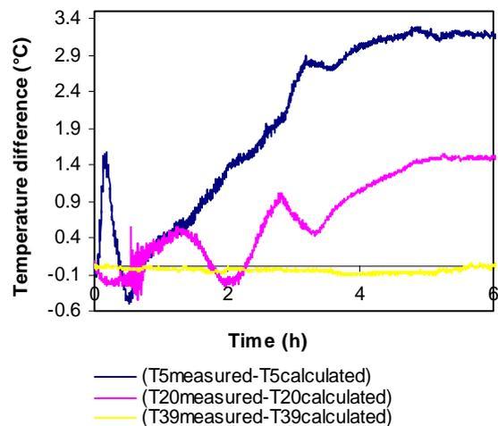
Figure 9 Differences between the three temperatures calculated and measured in the storage tank for injection of the fluid at different levels in the mantle with electric supply.
