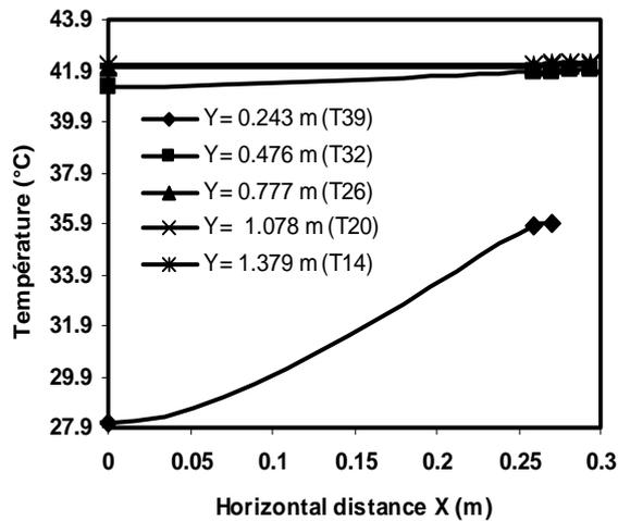
Figure 6 Compared temperatures according to X (radius) at different height levels of the tank.
