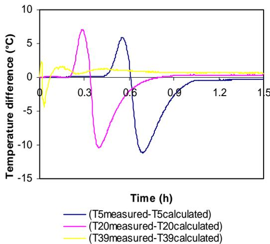
Figure 11 Differences between the three temperatures calculated and measured in the storage tank for a step of load flow rate
