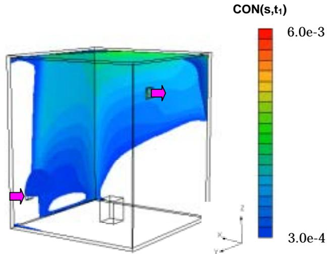
Figure 5 Predicted  $CON(s, t_1)$  contours for Case2 ( $t_1=60min$ )
