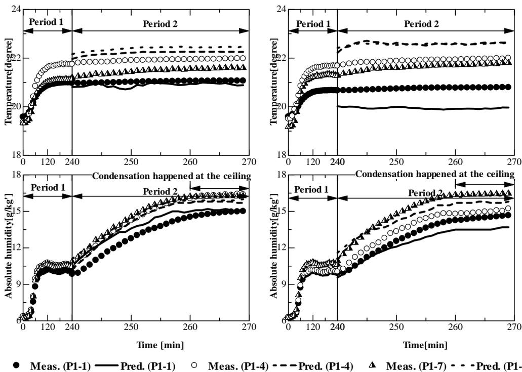
Figure 3 Comparison between measured and predicted temperature and moisture variations (Case1)
