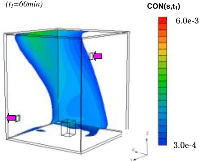
Figure 6 Predicted  $CON(s, t_1)$  contours for Case3 ( $t_1=60min$ )
