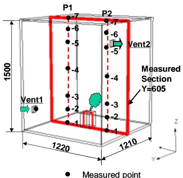
Figure 1: Schematic of the validation experiment within a test chamber (Unit: mm)
