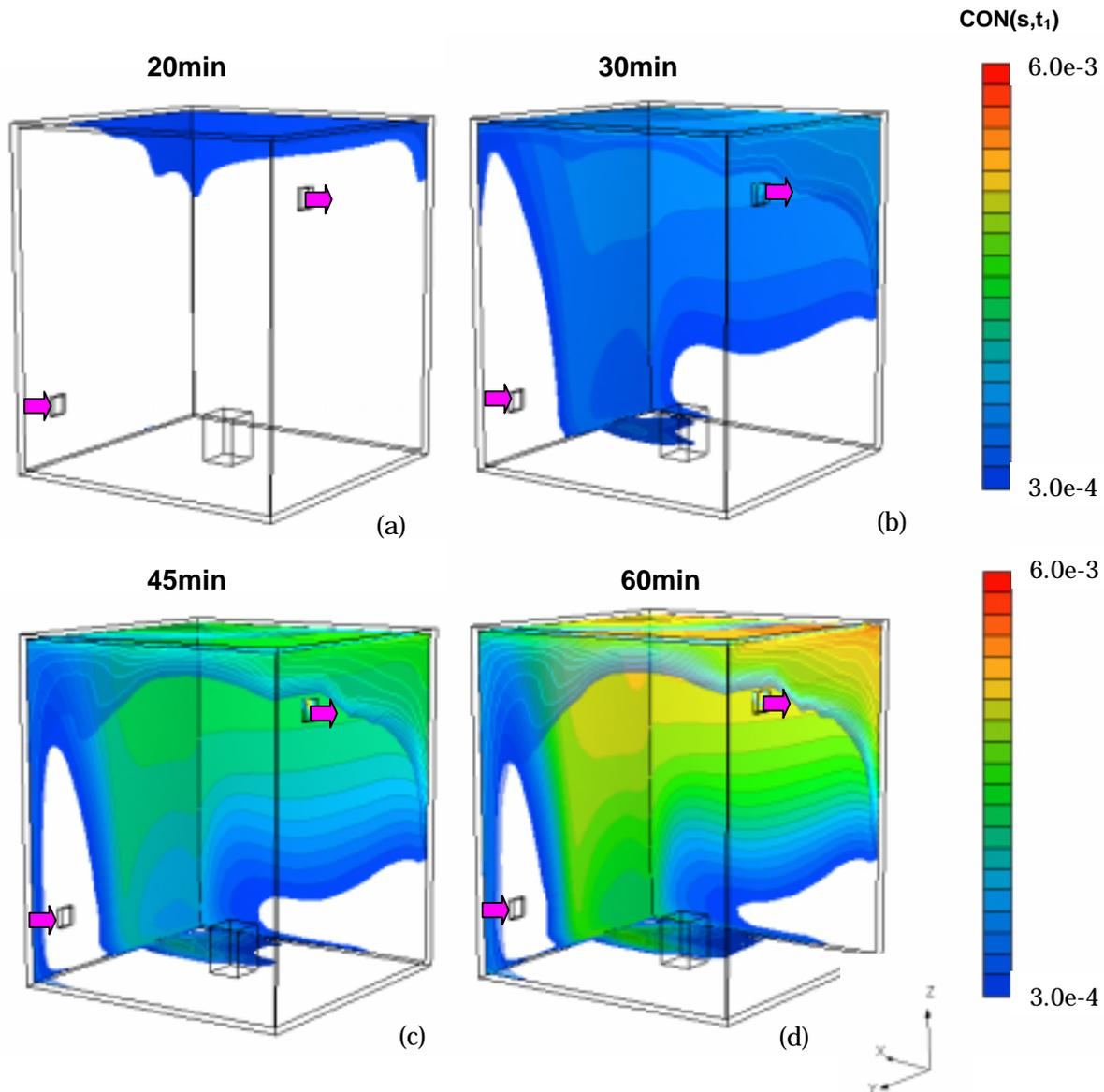
Figure 4 Predicted  $CON(s, t_1)$  contours for Case 1
