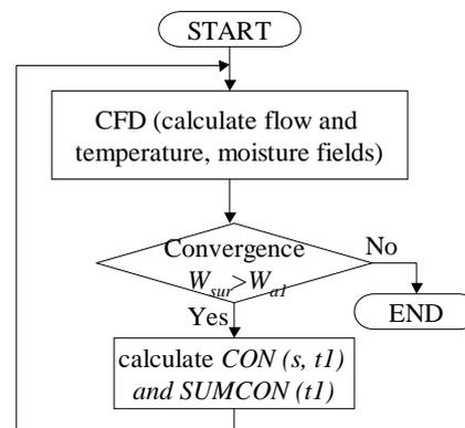
Figure 2 Flow chart of combined simulation of airflow, moisture and condensation
