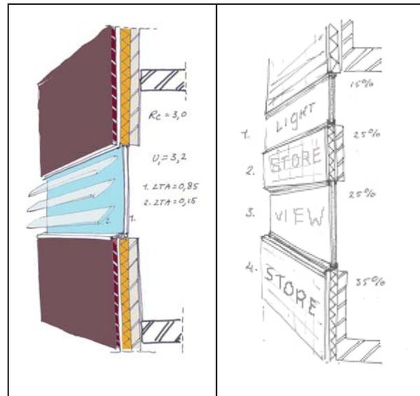
Table 1: Different variants for the insulation of the daylight and view opening
