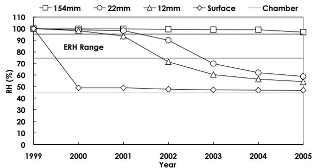
Figure 16 Interstitial RH at four vault depths
