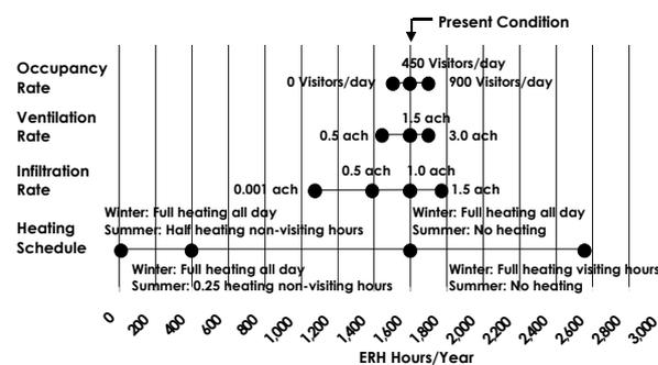
Figure 12 ERH sensitivity under varying internal condition
