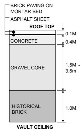
*Figure 2 Cross section of the brick vault*
