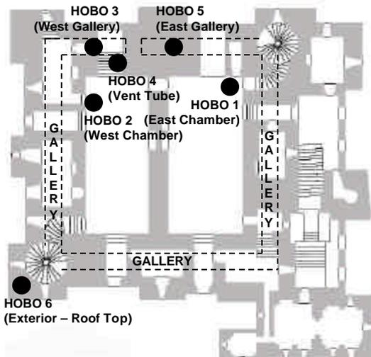
Figure 4 First floor plan with datalogger locations indicated
