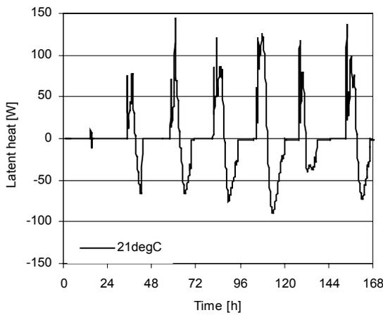
Figure 4. Solar energy stored as a latent heat in PCM-composite wallboard ( $T_m=21\text{ }^\circ\text{C}$ ).
