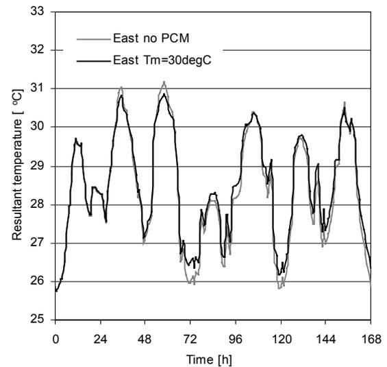
Figure 17. Resultant temperature history in east zone with traditional (no PCM) and PCM ( $T_m=27\text{ }^\circ\text{C}$ ).
