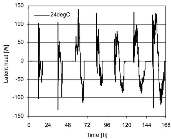
Figure 10. Solar energy stored as a latent heat in PCM-composite wallboard ( $T_m=27^\circ\text{C}$ ).
