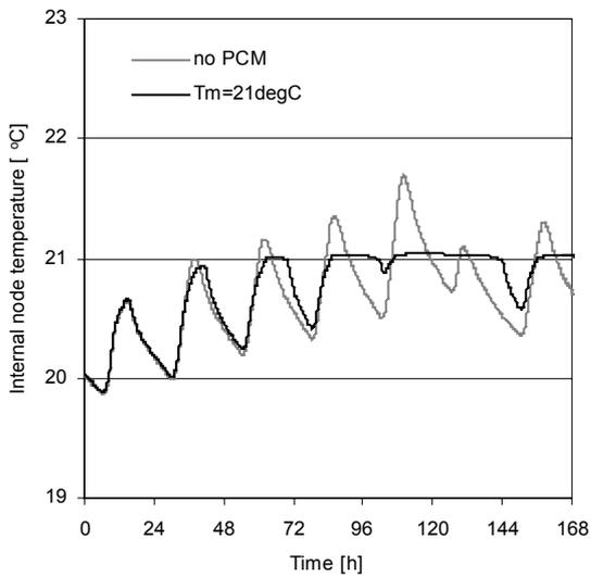
Figure 3. Internal node temperature history with traditional (no PCM) and PCM ( $T_m=21\text{ }^\circ\text{C}$ ).
