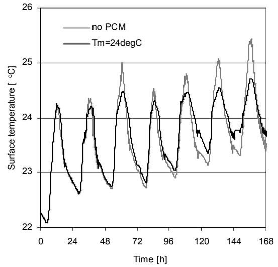
Figure 5. Wallboard surface temperature history with traditional (no PCM) and PCM ( $T_m=24\text{ }^\circ\text{C}$ ).
