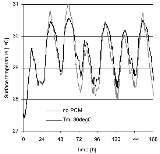
Figure 11. Wallboard surface temperature history with traditional (no PCM) and PCM ( $T_m=30^\circ\text{C}$ ).
