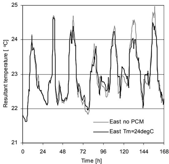
Figure 15. Resultant temperature history in east zone with traditional (no PCM) and PCM ( $T_m=24\text{ }^\circ\text{C}$ ).
