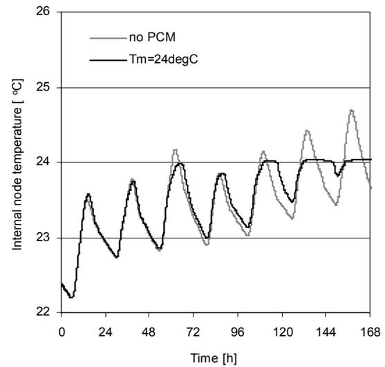
Figure 6. Internal node temperature history with traditional (no PCM) and PCM ( $T_m=24\text{ }^\circ\text{C}$ ).
