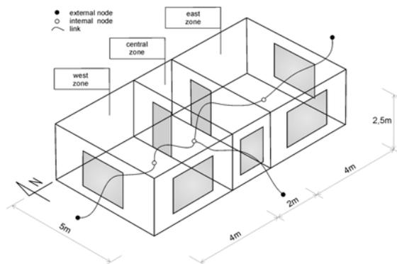
Figure 1. View of the 3 zones PCM building model.
