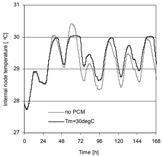
Figure 12. Internal node temperature history with traditional (no PCM) and PCM ( $T_m=27^\circ\text{C}$ ).
