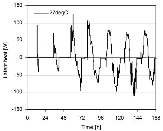
Figure 7. Solar energy stored as a latent heat in PCM-composite wallboard ( $T_m=24\text{ }^\circ\text{C}$ ).
