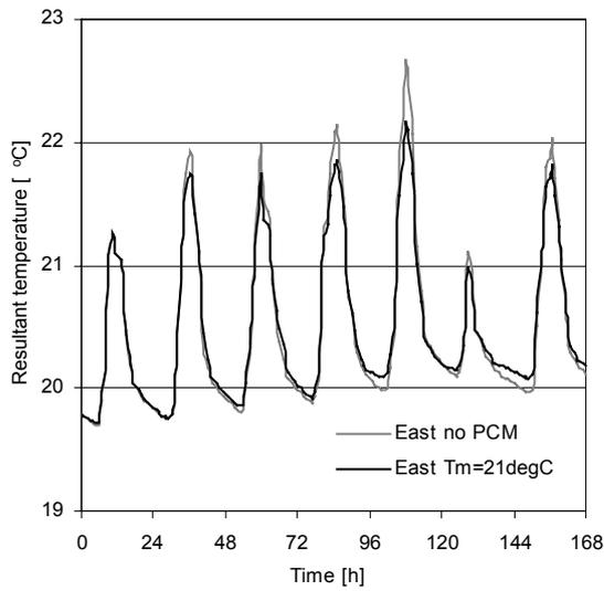
Figure 14. Resultant temperature history in east zone with traditional (no PCM) and PCM ( $T_m=21\text{ }^\circ\text{C}$ ).
