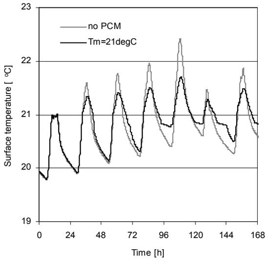
Figure 2. Wallboard surface temperature history with traditional (no PCM) and PCM ( $T_m=21\text{ }^\circ\text{C}$ ).
