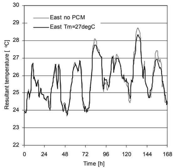
Figure 16. Resultant temperature history in east zone with traditional (no PCM) and PCM ( $T_m=27\text{ }^\circ\text{C}$ ).
