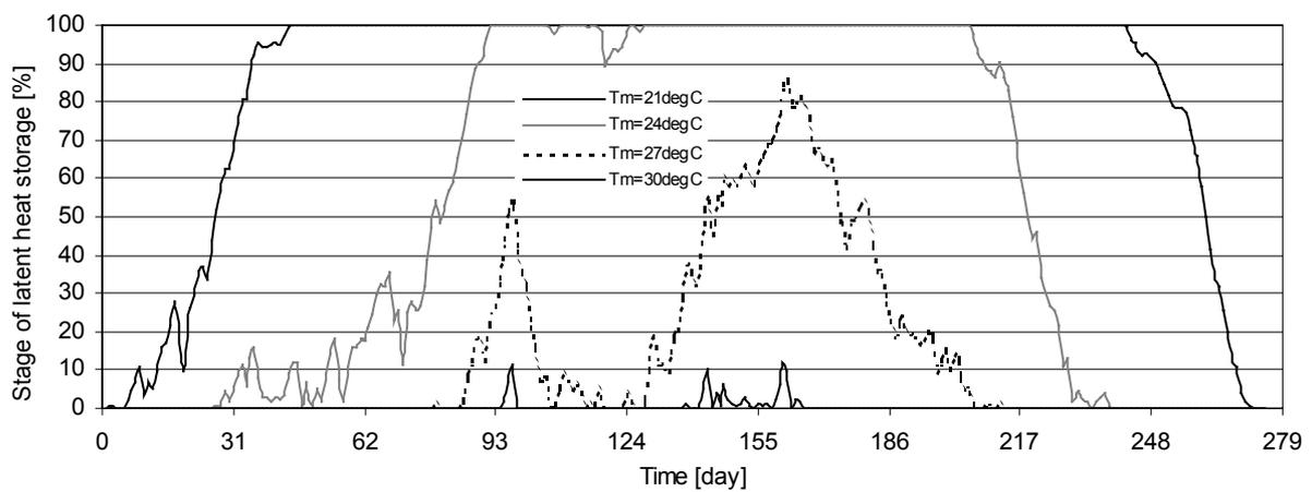
Figure 18. Latent heat storage stage for PCM-composites with different melting temperature from beginning of March to the end of November.
