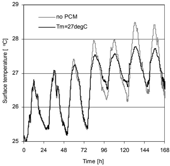
Figure 8. Wallboard surface temperature history with traditional (no PCM) and PCM ( $T_m=27^\circ\text{C}$ ).
