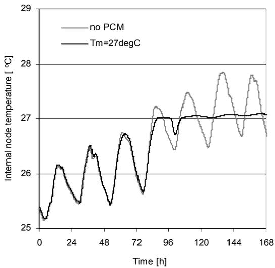
Figure 9. Internal node temperature history with traditional (no PCM) and PCM ( $T_m=27^\circ\text{C}$ ).
