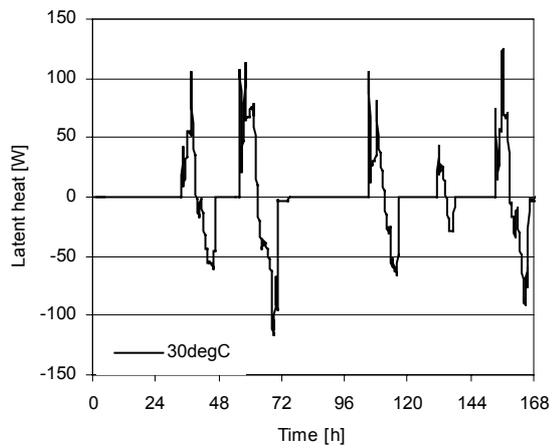
Figure 13. Solar energy stored as a latent heat in PCM-composite wallboard ( $T_m=30^\circ\text{C}$ ).
