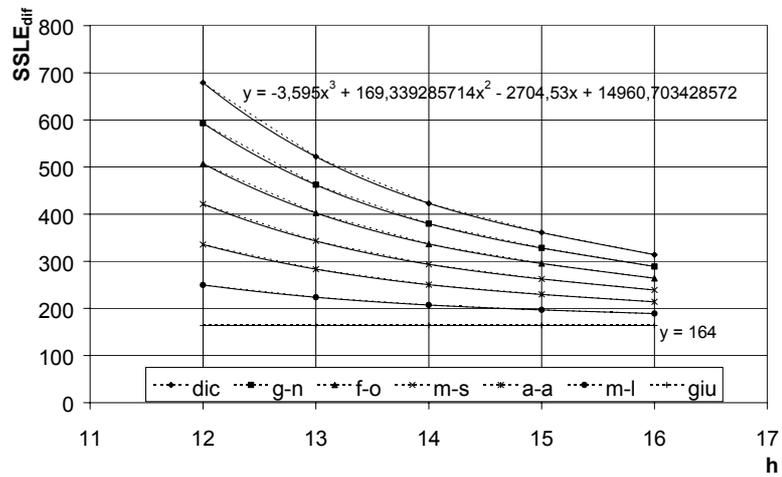
Figure 3.  $SSLE_{diff}$  for South orientation, 1.0m external overhang.
