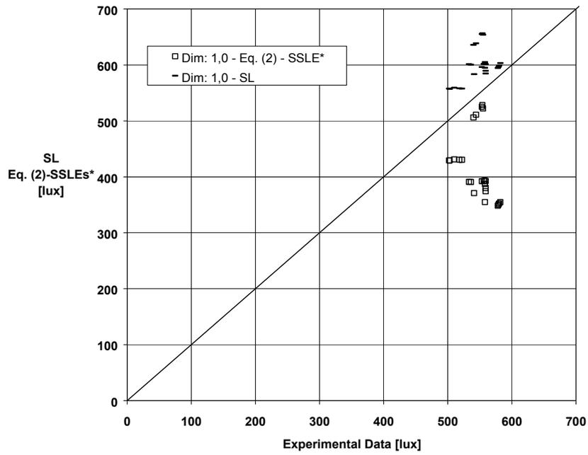
Figure 1: Scale model measurements versus Superlite (SL) and Equation (2) with SSLEs\* calculations, 1.0m external overhang.
