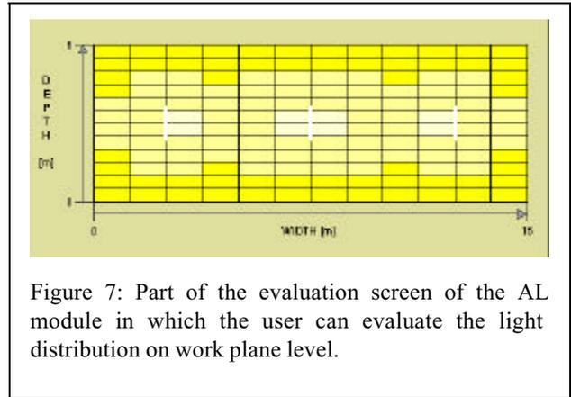
Figure 7: Part of the evaluation screen of the AL module in which the user can evaluate the light distribution on work plane level.
