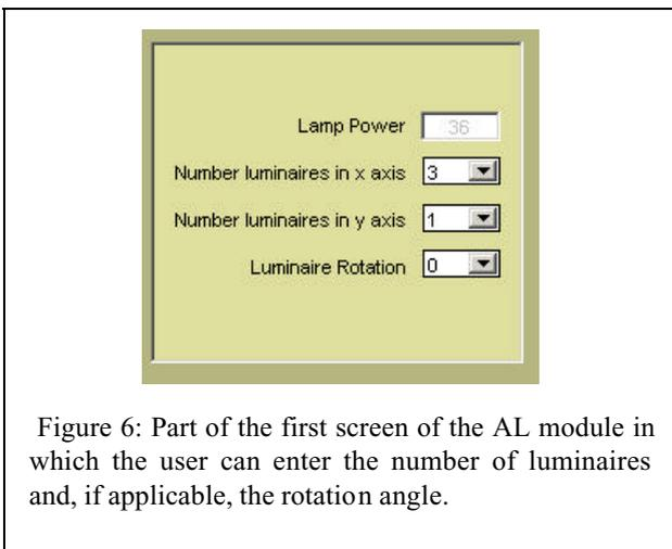
Figure 6: Part of the first screen of the AL module in which the user can enter the number of luminaires and, if applicable, the rotation angle.
