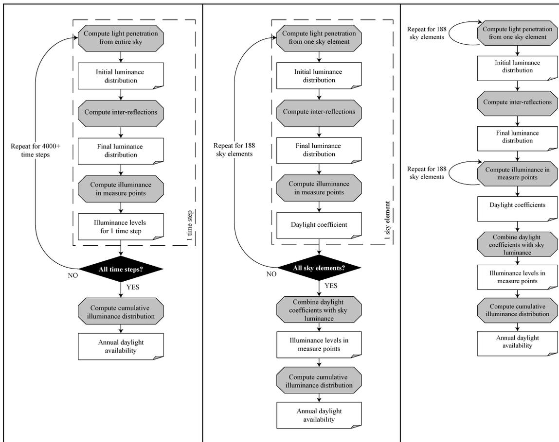
Figure 3. Flowcharts representing three methods for performing long-term daylight availability predictions while taking the daylight condition of each individual time step into account: one simulation per time step (left), one simulation per daylight coefficient (middle), parallel computation of daylight coefficients (right).
