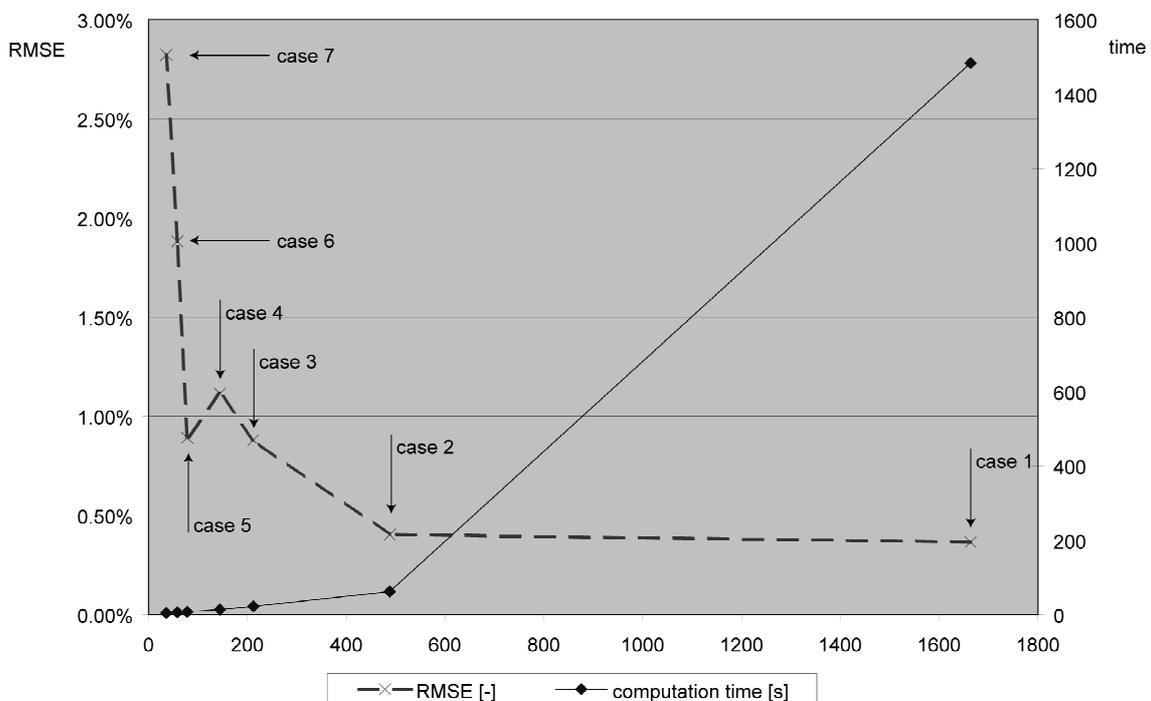
Figure 2. The RMSE of the total daylight factor and the computation time as function of the number of patches in the scene. RMSE is in percent of the total DF; computation time is in seconds.
