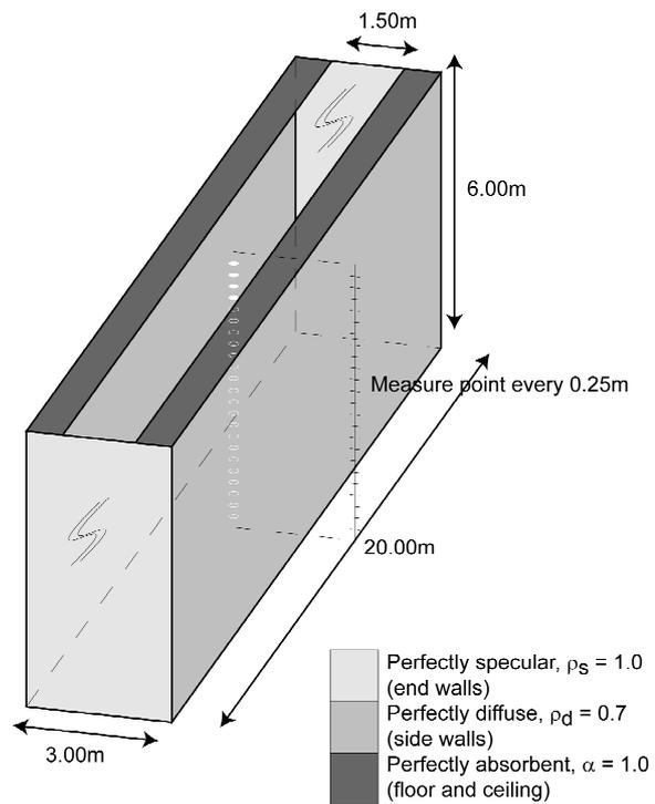
Figure 1. The experimental model to assess the impact of surface patch size on numerical accuracy.
