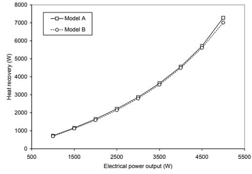
Figure 8: Model heat recovery estimates at reduced cooling water inlet temperature ( $T_{cw_i} = 55^\circ\text{C}$ ,  $\dot{V}_{cw} = 0.15\text{ l/s}$ )
