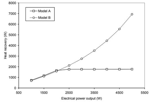
Figure 9: Model heat recovery estimates at increased cooling water inlet temperature ( $T_{cw_i} = 74^\circ\text{C}$ ,  $\dot{V}_{cw} = 0.15\text{ l/s}$ )
