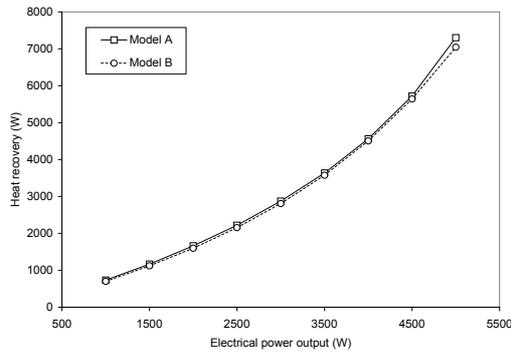
Figure 10: Model heat recovery estimates at increased cooling water flow rate ( $T_{cw_i} = 65^\circ\text{C}$ ,  $\dot{V}_{cw} = 0.17\text{ l/s}$ )
