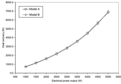
Figure 7: Model heat recovery estimates under design conditions ( $T_{cw_i} = 65^\circ\text{C}$ ,  $\dot{V}_{cw} = 0.15\text{ l/s}$ )
