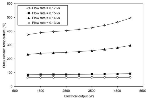
Figure 13: Model B exhaust gas outlet temperature response to changes in the cooling water flow rate
