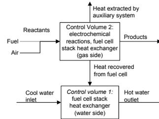
Figure 3: PEFC component model (Model A)
