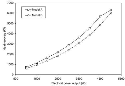
Figure 11: Model heat recovery estimates at reduced cooling water flow rate ( $T_{cw_i} = 65^\circ\text{C}$ ,  $\dot{V}_{cw} = 0.13\text{ l/s}$ )
