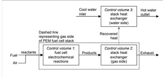
Figure 5: Adaptation of Model B to represent PEFC stack
