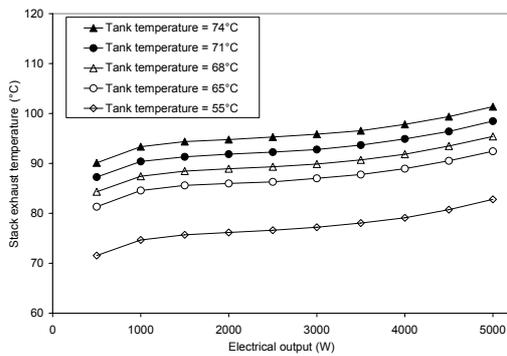
Figure 12: Model B exhaust gas outlet temperature response to changes in the cooling water inlet temperature
