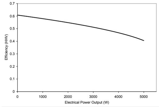
Figure 2: Test case part-load electrochemical performance
