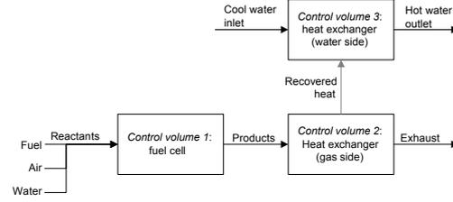
Figure 4: SOFC component model (Model B)
