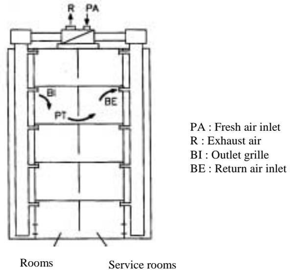
Figure 6 : Principle of dual flow ventilation system
