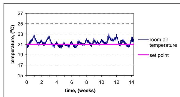
Figure 2 : Room air temperature. Above: heating curve was not adjusted (case 1a in Table 1). Below: heating curve was adjusted automatically (case 1b in Table 1).
