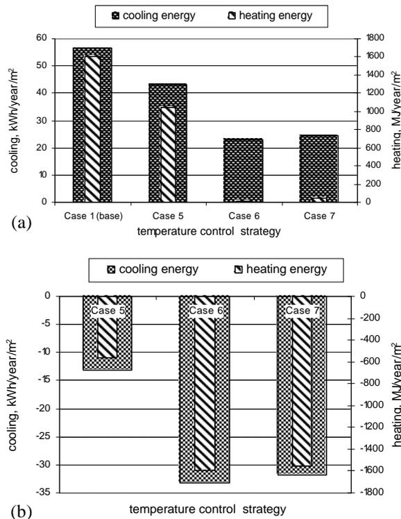
Figure 2 Change in annual cooling and heating energy requirements at different temperature control strategies; (a) relative variations, (b) magnitude of change (relative to base case)
