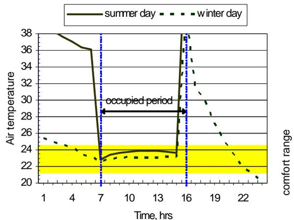
Figure 7 Indoor temperature variations when temperature control starts one hour prior to occupancy and ends one hour before the end of occupancy
