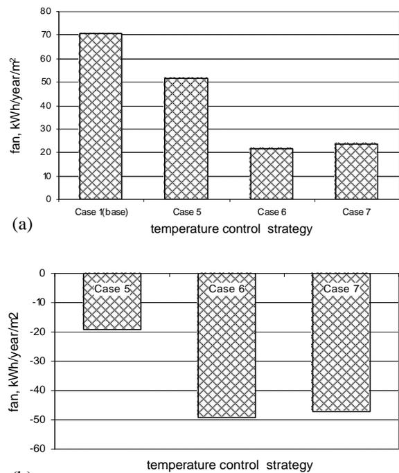
Figure 3 Change in annual fan energy requirements at different temperature control strategies; (a) relative variations, (b) magnitude of change
