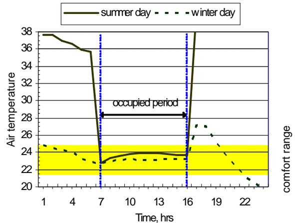
Figure 6 Indoor temperature variations when temperature control starts one hour prior to occupancy
