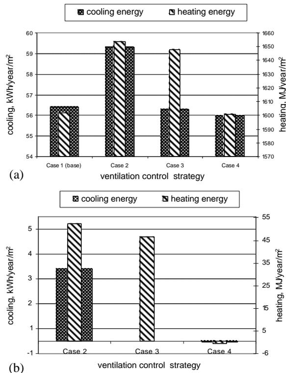
Figure 1 Change in annual cooling and heating energy requirements at different ventilation control strategies; (a) relative variations, (b) magnitude of change (relative to base case)
