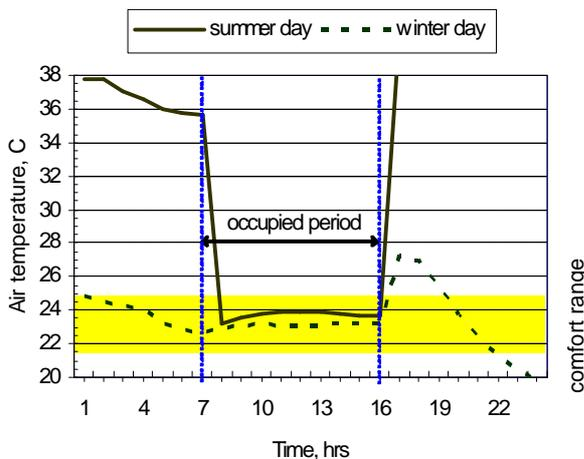
Figure 5 Indoor temperature variations when temperature control is limited to the occupied period
