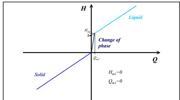
Figure 3 Relation between the enthalpy without dimension and the temperature without dimension.
