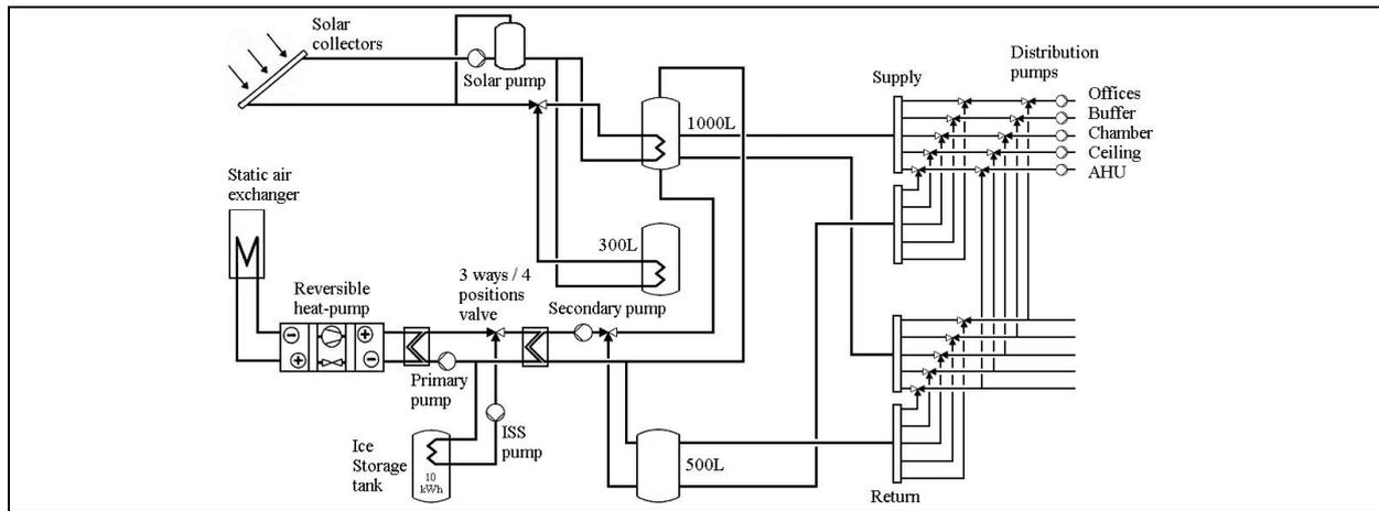
Figure 5 Test bench scheme
