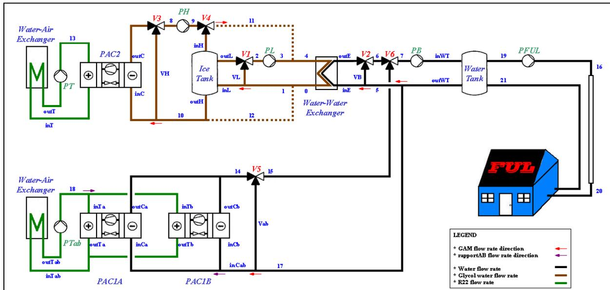
Figure 7 Scheme of the primary HVAC plant of FUL building
