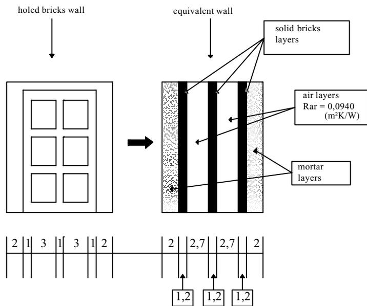
**Figure 6 - Equivalent wall**
