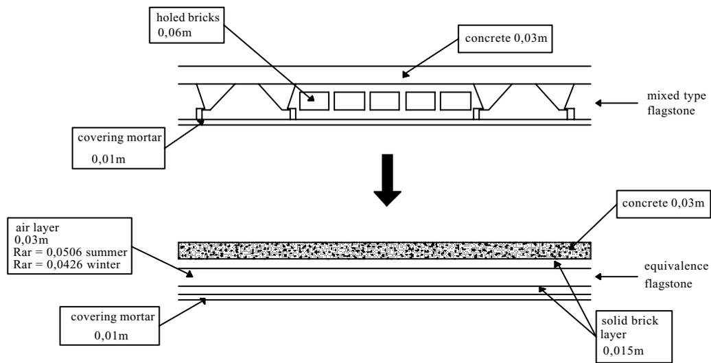
**Figure 7 – Equivalence of mixed type flagstone coverings**
