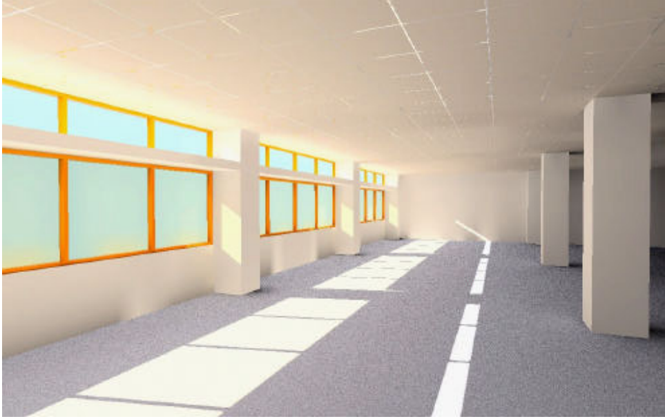
Figure 6: Rendering of daylight penetration with articulated glazing and light shelf on a typical south facade, 12:00 PM on December 21st (no furniture).
