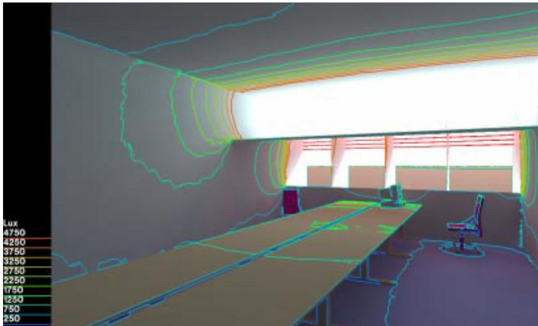
Figure 4c: False color image for light shelf with fins, 21<sup>st</sup> of June, CIE clear sky sun
