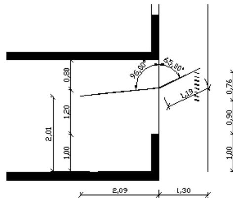
Figure 1: section of type room with light shelves, fins and glare protection
