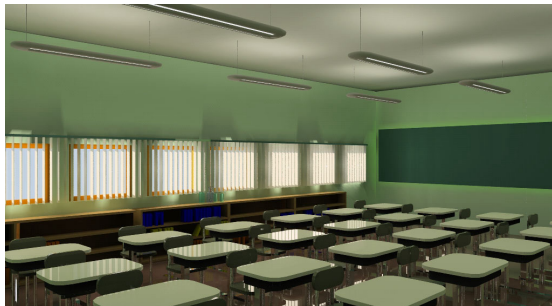
Fig. 6 Radiosity solution and ray tracing from Lightscape.
