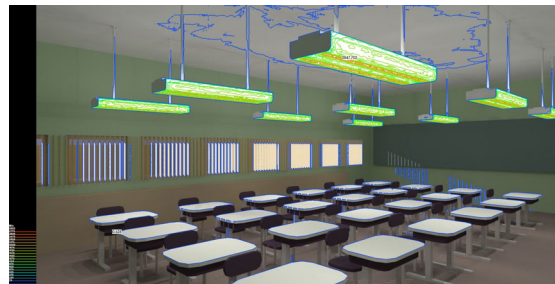
Fig. 8 Luminance analysis with contour lines (Radiance)
