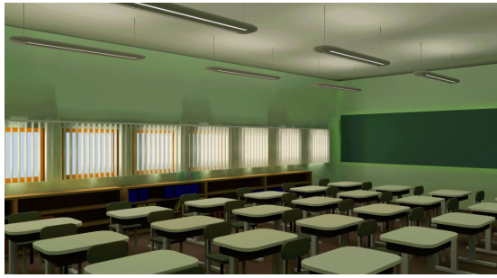
Fig. 5 Radiosity solution from Lightscape.
