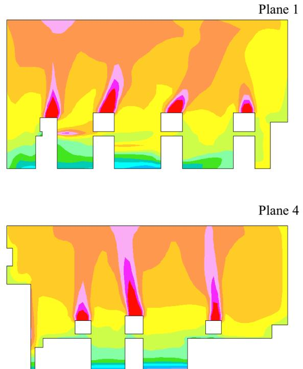
Fig. 8 Temperature field in the vertical planes 1 and 4 for Variant I
