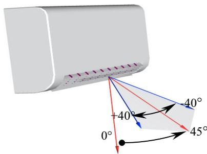
Fig.2 Schematic view of A/C diffuser
