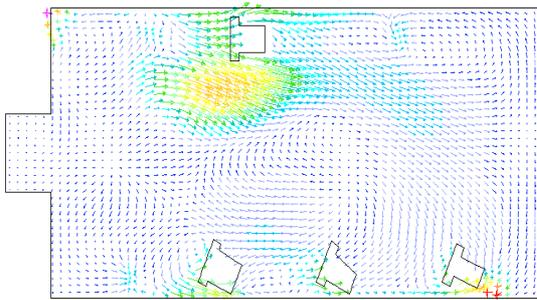
Fig. 13 Velocity field in the horizontal plane 5 - variant IV.A
