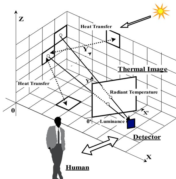
Fig. 1. Generating process of thermal image
