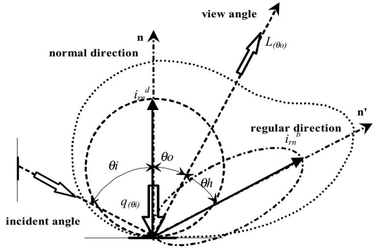
Fig. 5. Reflective luminosity model
