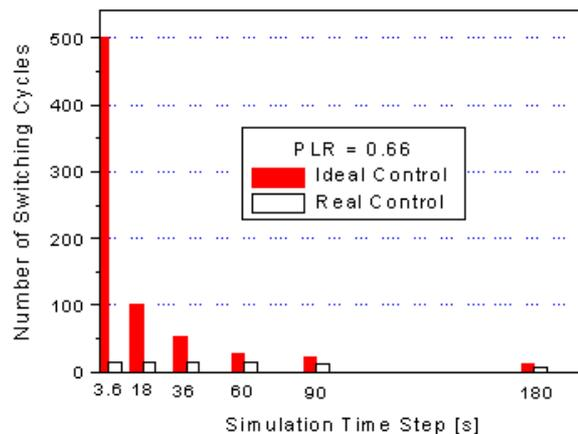
**Figure 5:** Maximum Number of Switching Cycles of the Compressor at Different Time Steps within 2 Hours of Simulation
