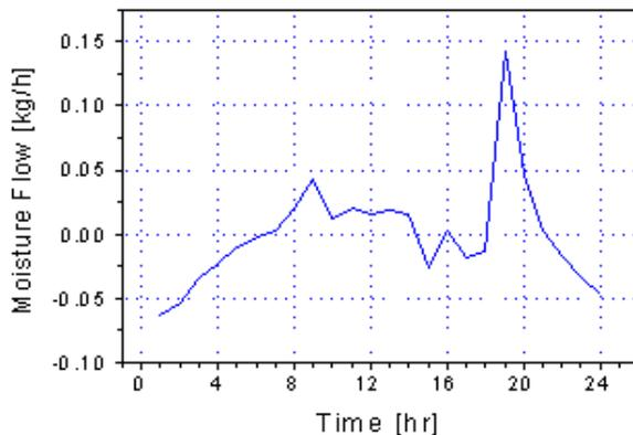
**Figure 17:** Total Moisture Flow through Adsorption and Absorption of the Interior Plaster
