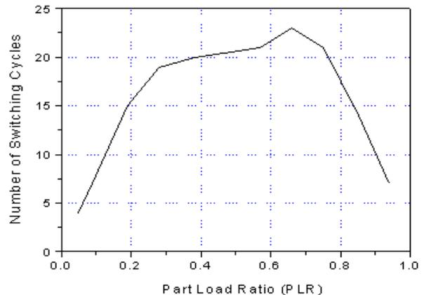
**Figure 4:** Number of Switching Cycles of the Compressor Depending on PLR at a Time Step of 90 s within 2 Hours of Simulation
