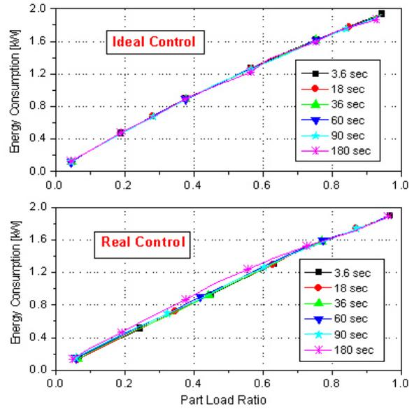
**Figure 8:** Total Energy Consumption at Different Kinds of Control. Compressor and Supply Fan Cycle Together.
