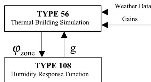
**Figure 2:** Coupling Scheme in TRNSYS
