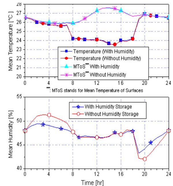
Figure 16: Results of two Cases: With and Without Humidity Storage in the Walls
