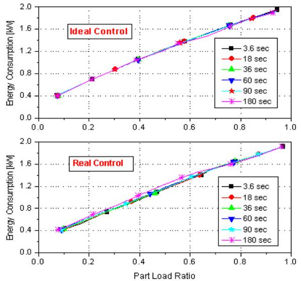
**Figure 9:** Total Energy Consumption at Different Kinds of Control, the Supply Fan Running Continuously.
