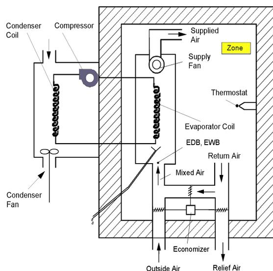
**Figure 1:** Scheme of the applied split system[4]
