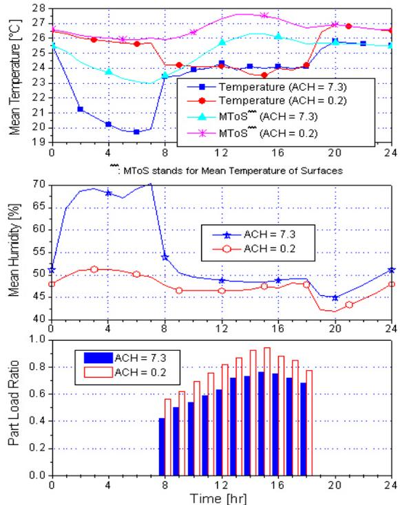
Figure 13: Results of Different Air Exchanges at Night
