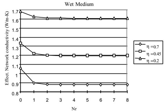
Figure 3: Effective thermal conductivity -  $\lambda_{ef}$  – as a function of step numbers of the renormalization process for a wet medium with  $\lambda_s=2$  W/m-K.
