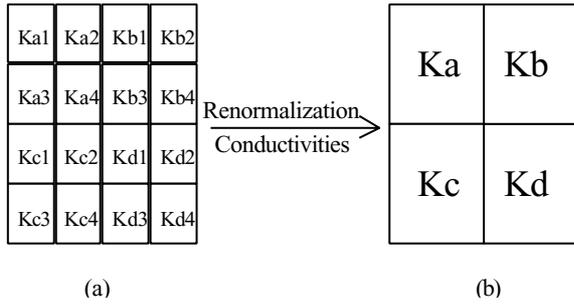
Figure 1. In (a) the original network of conductivities. In (b) the renormalized network with the effective conductivities.
