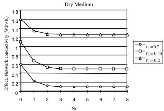
Figure 2: Effective thermal conductivity -  $\lambda_{ef}$  – as a function of step numbers of the renormalization process for a dry medium with  $\lambda_s=2$  W/m-K.
