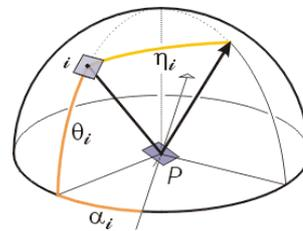
Fig. 5. Required angles to compute the illuminance of the centre  $P$  of a scene patch, collected from a sky patch  $i$ .  $\alpha_i$  and  $\theta_i$  are the azimuth and altitude of the sky patch  $i$  respectively, and  $\eta_i$  the angle between the sky patch and the normal to the surface element of the scene containing point  $P$  (this angle is measured on a great circle of the hemisphere).
