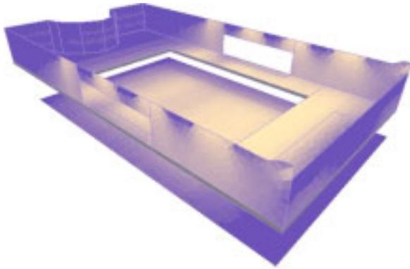
Fig. 17. The illuminance levels of the second floor show high values (around 3000 lux) near the waiting rooms.
