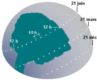
Fig. 22. Example of the sky area seen through a window, with superimposition of the solar paths.
