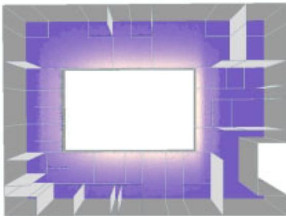
Fig. 19. Illuminance levels with an overcast sky on a 0.8 meter high working plane (our attention is now focused on the laboratories, so the patio is neither displayed on this picture nor on the following ones).
