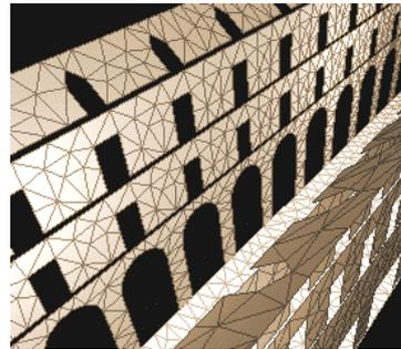
Fig. 4. A meshed urban street ; the size of the patches is adaptable and depends on the expected accuracy and the scale of the simulated environment.
