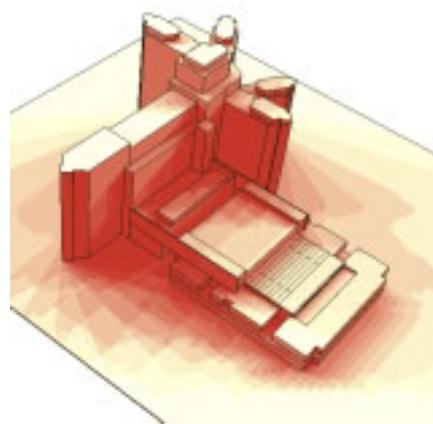
Fig. 15. Simulation of the duration of sunshine at equinoxes for the whole complex.
