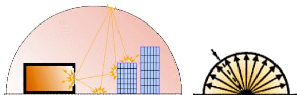
Fig. 7. Reflections on the different surfaces of the urban environment (*left*). Ideal diffuse reflection, which is equal in every direction (*right*).
