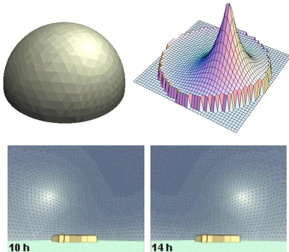
Fig. 3. Visualisation in SOLENE of the luminance distribution for a clear sky on the meshed hemisphere (1024 patches) ; each triangle is coloured according to its luminance value (top left). An alternate representation mode of the same sky with height fields (top right). Under the sky vault : two pictures of a one-hour step animation showing the displacement of the area of high luminance levels (bottom).
