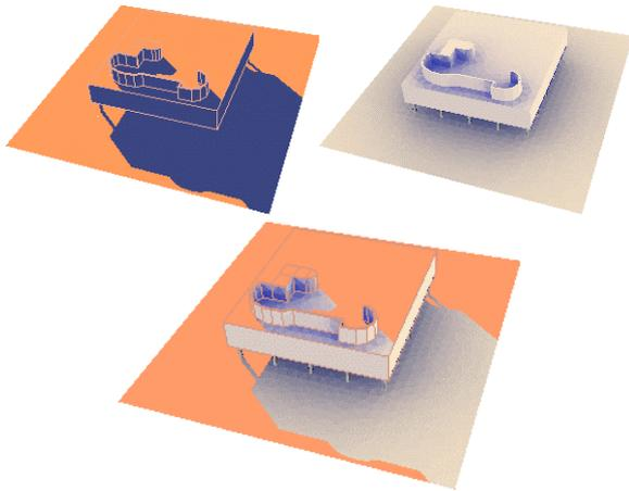
Fig. 6. A simulation of the Villa Savoye in SOLENE (sept. 21<sup>st</sup>, 10 h, clear sky) : The direct illuminance levels (*top left*) ; the illuminance levels due to the sky vault only (*top right*) ; the combination of the previous gives the illuminance levels of the entire meshed scene (*bottom*).
