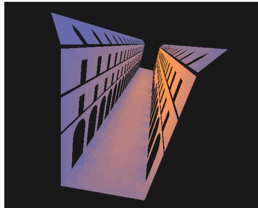
Fig. 13. Cartography of the contribution of the multi-reflexion process in the same street (difference between the illuminance levels after and before the process ; the luminance values are read in databases that are generated by the simulations and linked to the geometry file).
