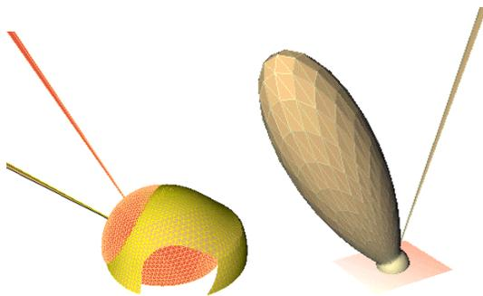
Fig. 24. Visualisation of BRDF with SOLENE : sheet of aluminium for different incidences (35 and 70°) with the Oren-Nayar model of reflectance [5] (left), and a polished marble (right) with a Cook-Torrance model.
