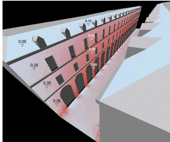
Fig. 12. The visualisation of the form factors in a urban street, displaying the importance of the middle area of the façades in the multi-reflexion process.
