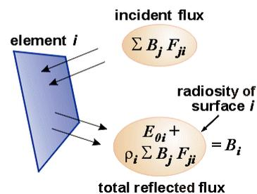
Fig. 9. Diagram of the radiative balance for a patch  $i$ .
