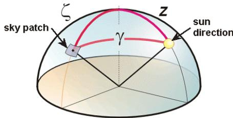
Fig. 2. The 3D geometry and angles required for the computation of the luminance of a sky patch of the zenithal altitude  $\zeta$ .
