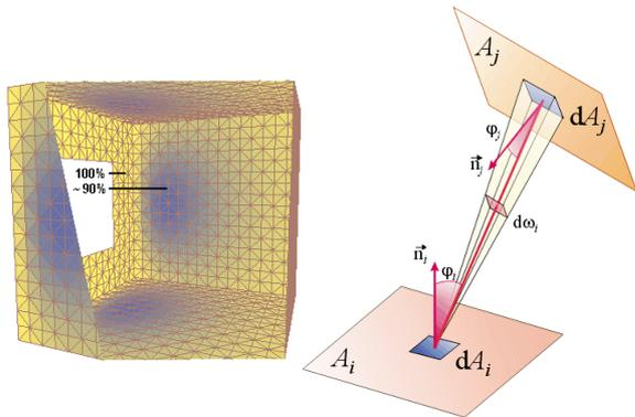
Fig. 11. The open architecture of SOLENE allows the visualisation of the form factors values (*left*). The geometry of form factors between two elements of surface (*right*).
