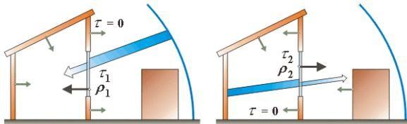
Fig. 14. Glazing is considered as an “ordinary” patch, but with an unsettled normal : it changes according to the direction of crossing.
