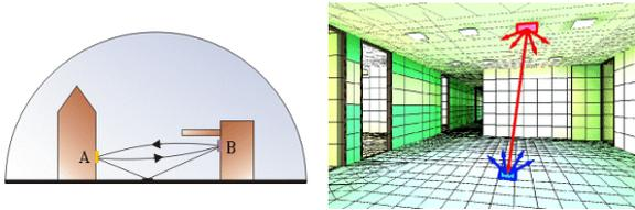
Fig. 10. Light interactions occur outdoor between surface elements of the urban environment (*bottom left*), and indoor (*bottom right*). One patch exchanges luminous energy with every other patch of the scene.
